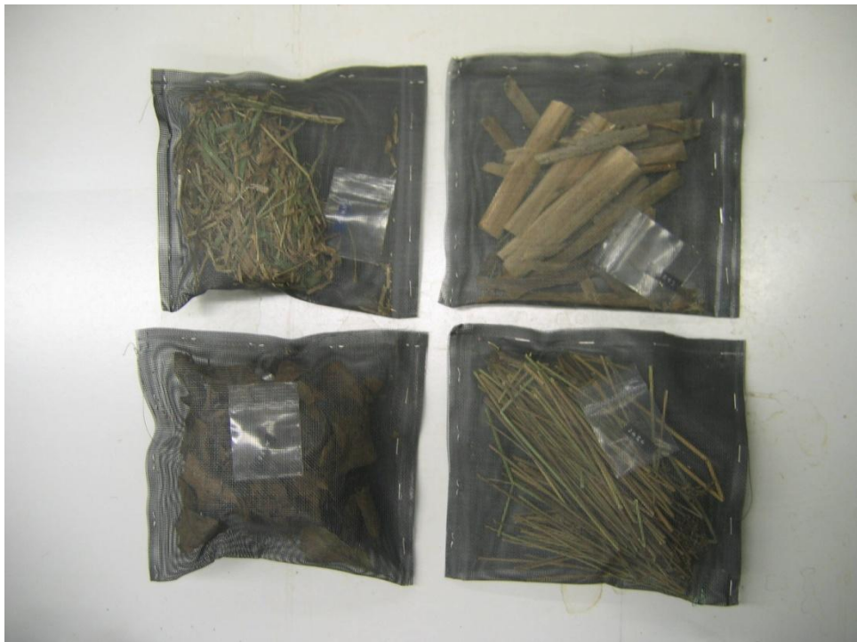
Figure 2. Photograph of the 4 single species (reed canary grass, broadleaf cattail, brookside alder, and common rush) litter bags with fine (1.27 mm) mesh.
