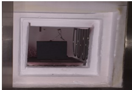
(b) Smart brick setup in furnace
