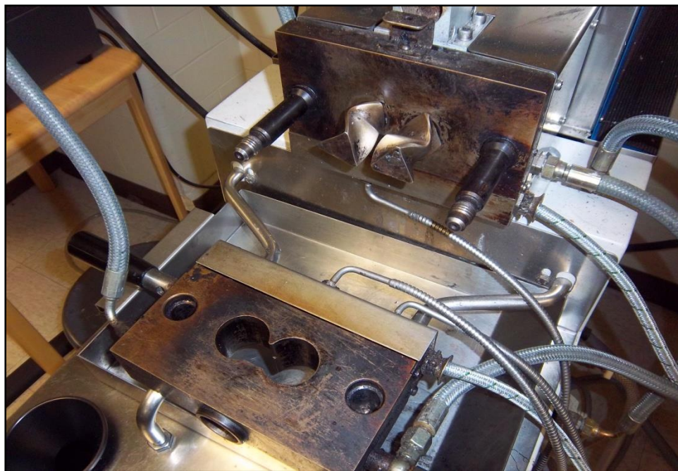
Figure 3.2: Internal mixer showing roller rotor blades.
