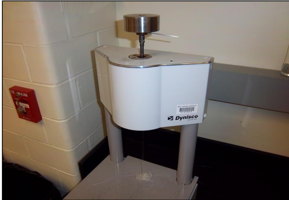
Figure 3.4: Melt flow indexer with piston and weight during test.
