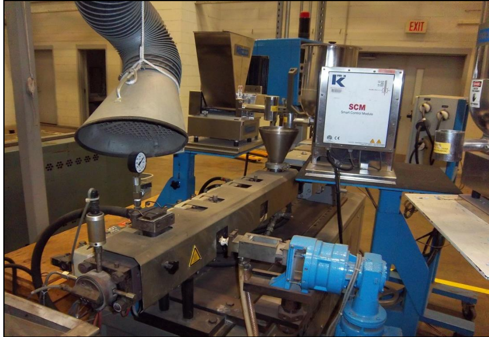
Figure 3.1: Leistriz 27 TSE with feeders, control box and vacuum trunk.
