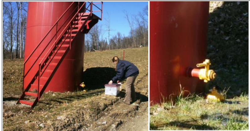
Figure 3.6 —Sampling flowback waters from holding tank. Close up of spigot from holding tank at shale gas drilling site (right). Samples were taken directly from the bottom being careful to minimize atmospheric exposure.
