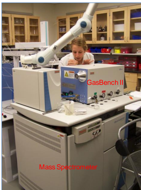
Figure 3.7 — GasBench II device coupled to a Finnigan Delta Plus mass spectrometer at the West Virginia Stable Isotope Laboratory.
