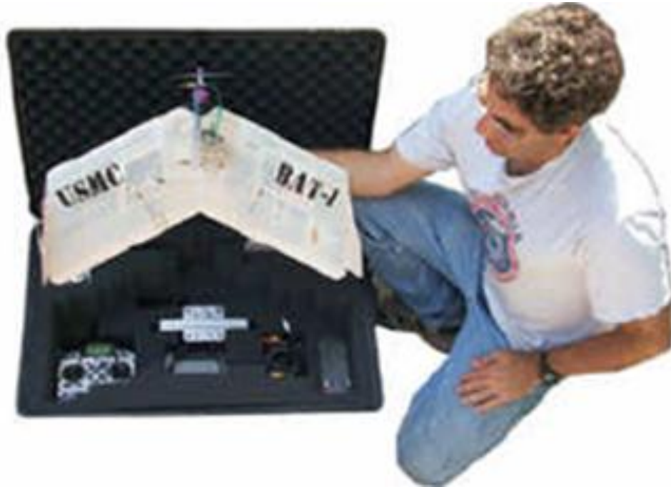
Figure 2-11: Ground Stations for MLB Bat MAV System (Morris, Design of Micro Air Vehicles and Flight Test Validation, 2000)
