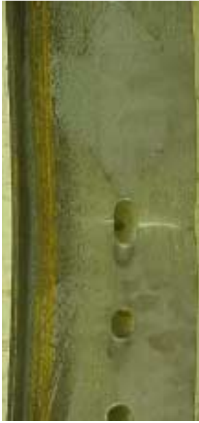
a: Partial net section rupture medium eccentricity b: Partial net section rupture large eccentricity
