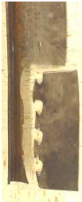
c: Block Shear Failure
