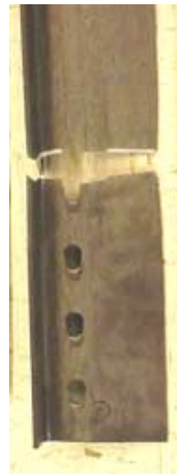
d: Full net section rupture failure
