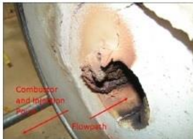
Figure 21: Image of large deposit formation on the left side of the transition piece [38]
