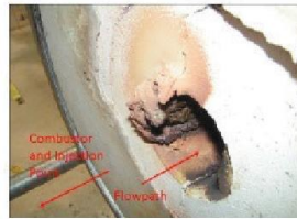
Figure 2. Image of large deposit formation on the left size of the transition piece [12].
