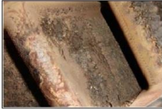
Figure 3: Film-cooled turbine vane covered by particulate matter from volcanic ash [8]
