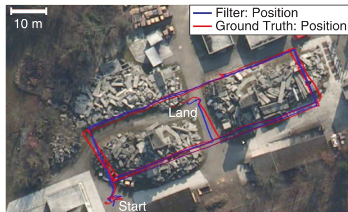
Figure 2.17: Vision Based Navigation using the camera-based position estimation. [14]
