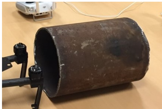
Figure 1.2: An eight inch pipe used for borehole casing
