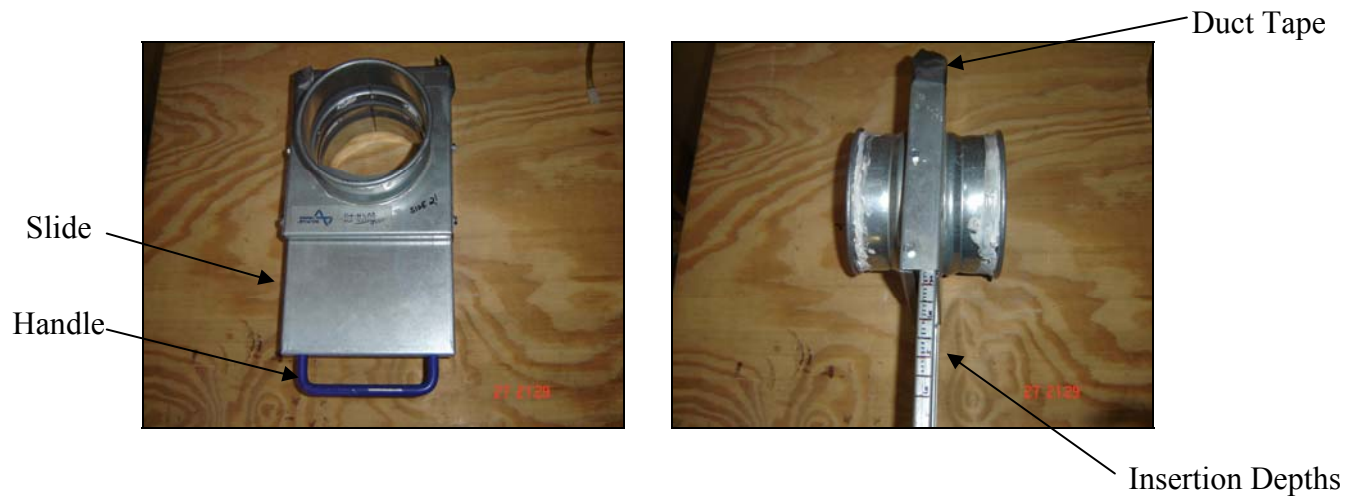
Figure 13 – Slide gate damper (Model No. 3241) used in the study
