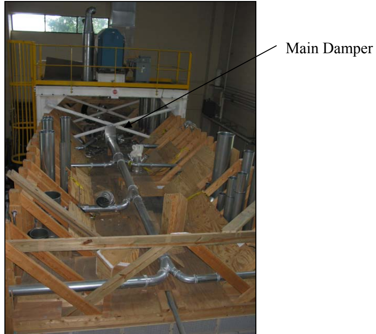
Figure 20 – Exhaust Ventilation System in Ventilation and Exposure Assessment Laboratory (WVU)
