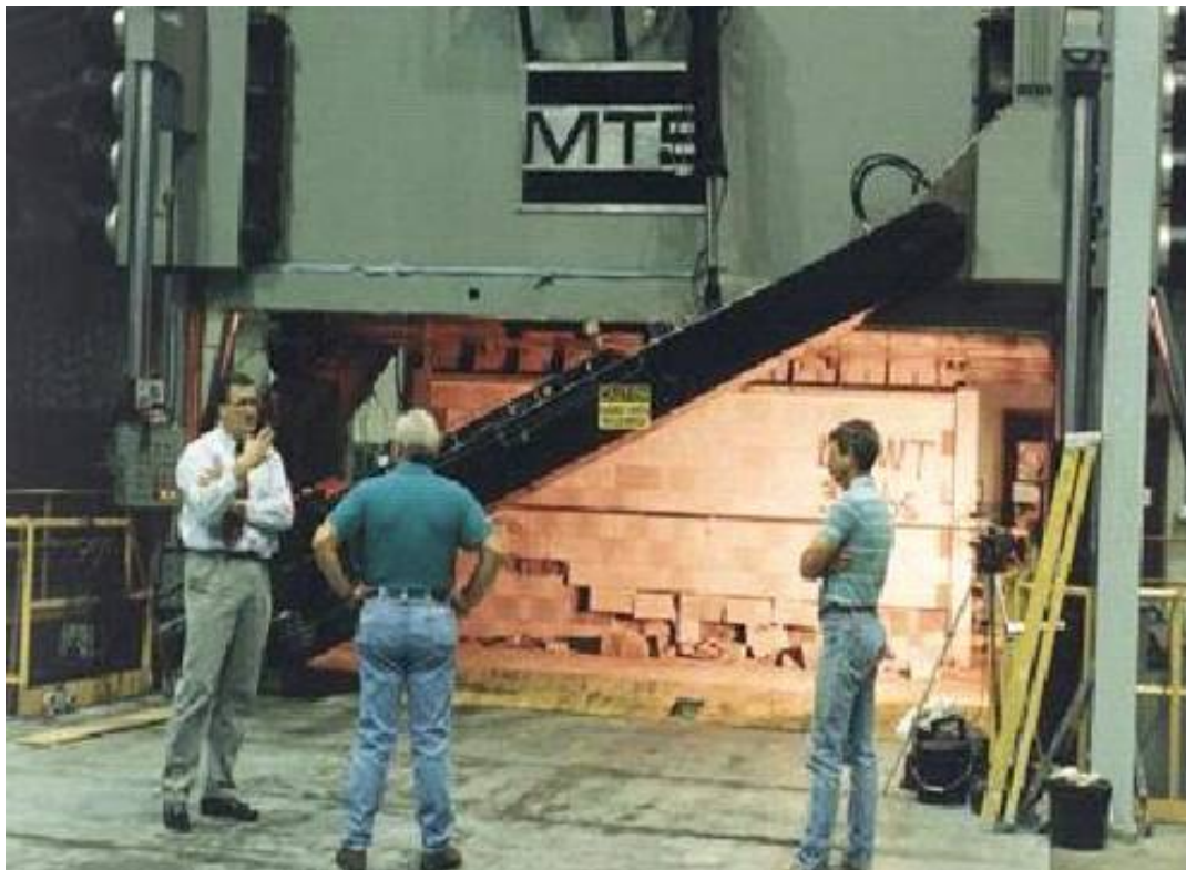
Figure 4-3. Full-scale mine ventilation stopping wall being tested in the NIOSH Mine Roof Simulator.
