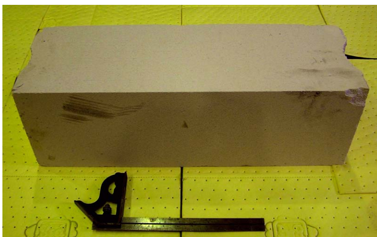
Figure 8-67. Ytong autoclaved aerated concrete block.
