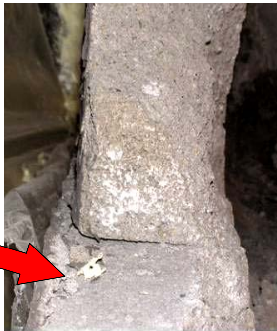
Figure 4-19. Close up view of the base of the conventional (Klondike) block wall showing the rotation of the wall and formation of the bottom hinge of the arch.
