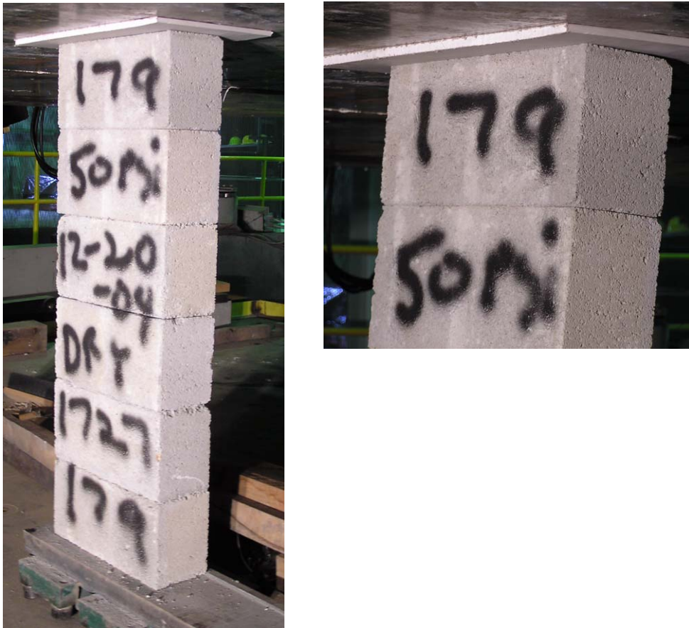
Figure 6-11. Test configuration using drywall to soften the abutment stiffness.
