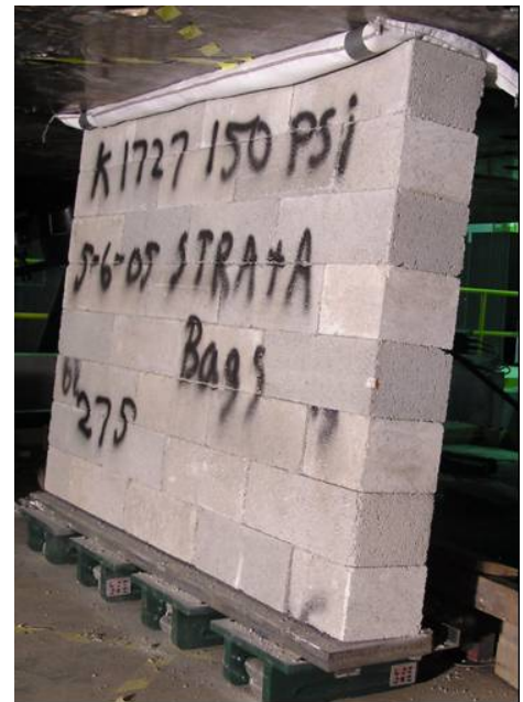
Figure 6-31. Testing of a half-wall with grout bag in the Mine Roof Simulator.
