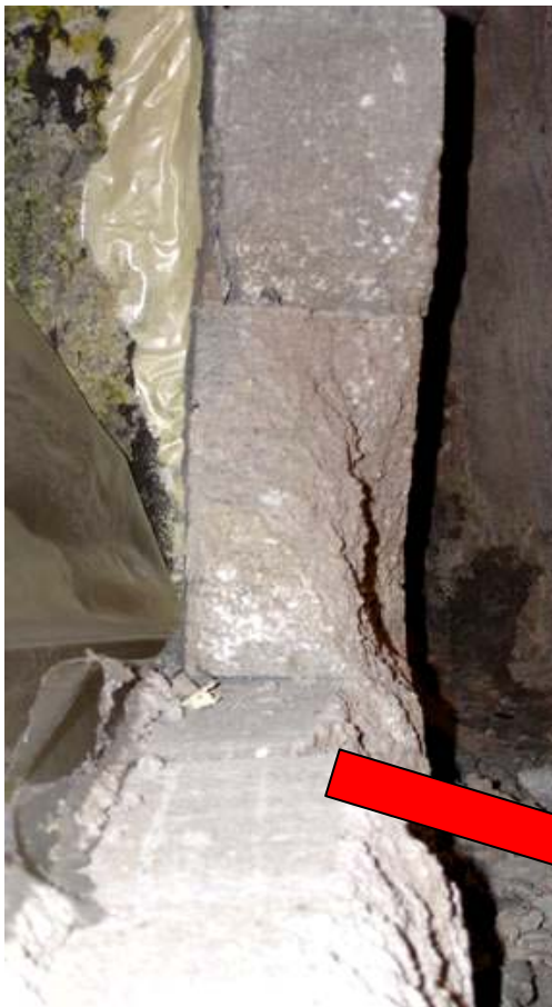
Figure 4-18. Photo showing conventional (Klondike) wall after full-scale test in the Experimental Coal Mine noting the arch length between the top and bottom course of block.
