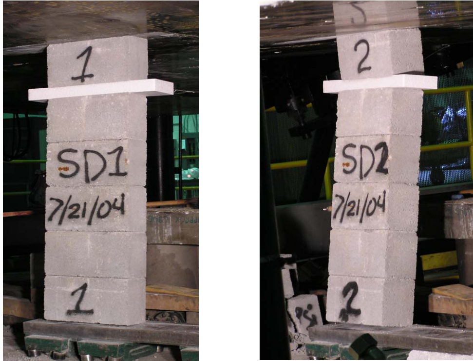
Figure 6-21. Half-walls with foam between the top two blocks shown with 3 inches of lateral displacement (left) and 7 inches of lateral displacement (right).
