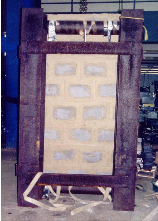
Figure 3-2. A 4 x 8 ft section of wall being placed into reaction frame for ASTM E 72 testing.
