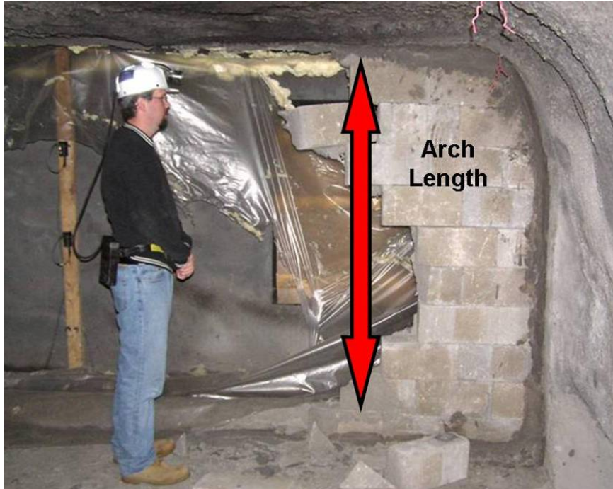
Figure 4-18. Photo showing conventional (Klondike) wall after full-scale test in the Experimental Coal Mine noting the arch length between the top and bottom course of block.
