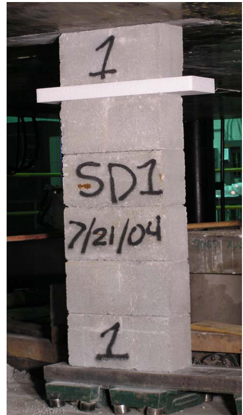
Figure 6-18. Half-wall test in the MRS with 2-inch-thick foam plank placed between the top two blocks.
