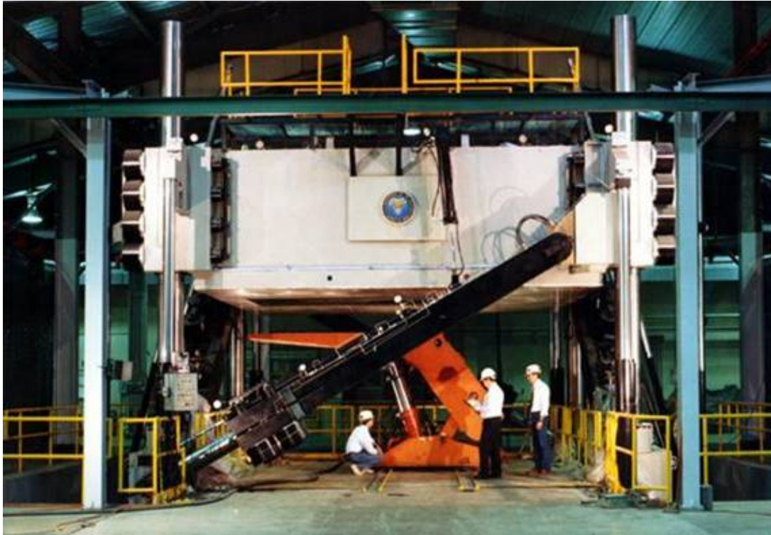
Figure 4-2. NIOSH Mine Roof Simulator load frame.
