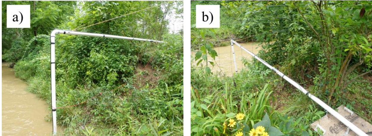
Figure 4. a) Front view of the SL3000 mount arm and b) rear view of the SL3000 mount arm
