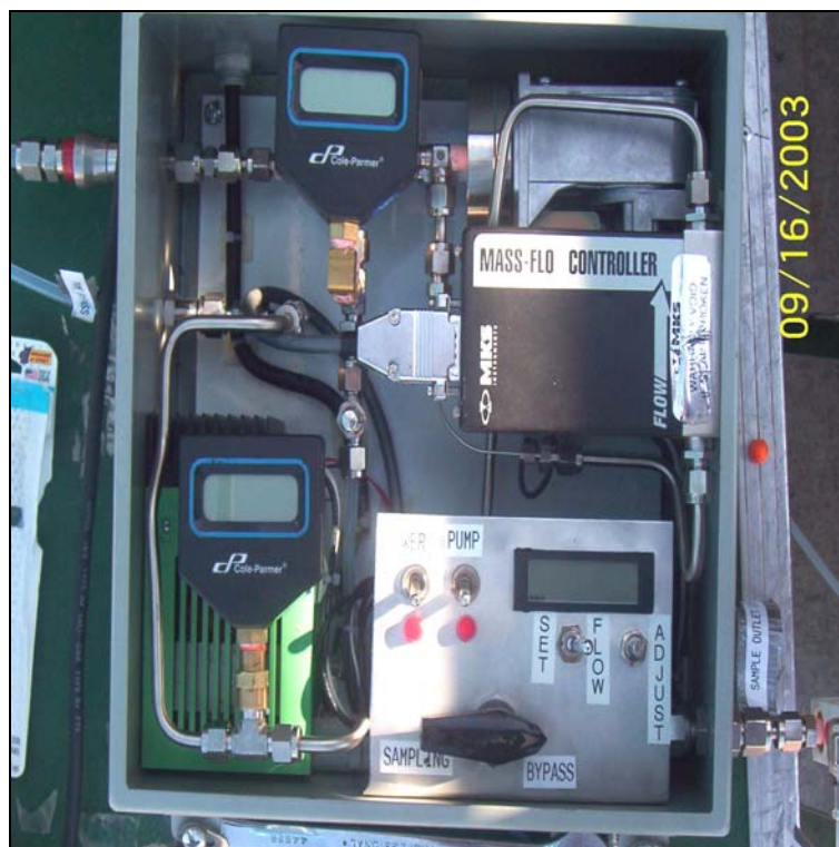
Figure 3.8 Volatile Organic Carbons Canister Sampling System.
