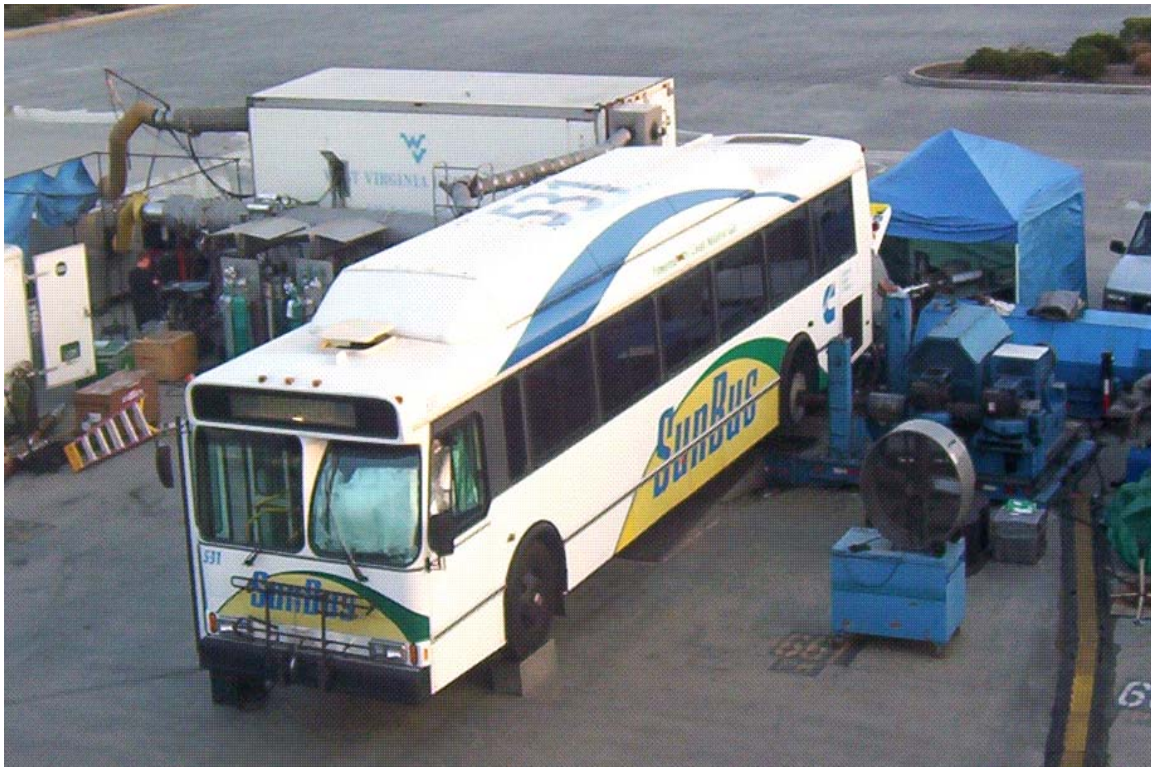
Figure 4.1 Test vehicle mounted on the chassis dynamometer
