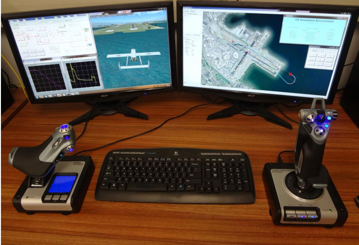
Figure 3. User interface with the UAV simulation environment.
