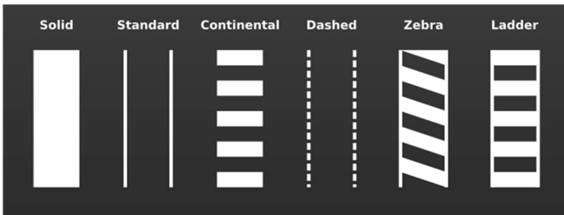
Figure 2.5-2: Crosswalk Pavement Markings
