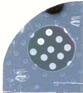
Figure 2-13: A typical sample for CV measurements. Small circular pads are aluminum top contacts.
