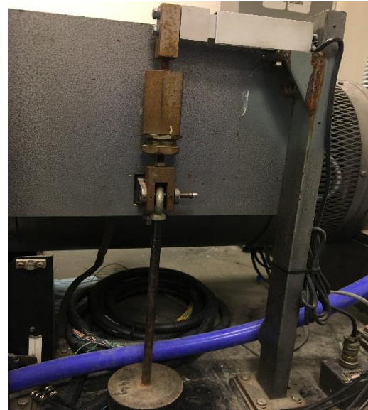
Figure 7: Load cell with hanger
