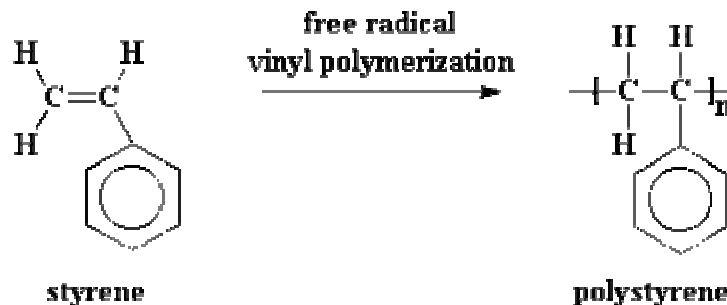
Figure B5: Polymerization of Styrene monomer to Polystyrene
