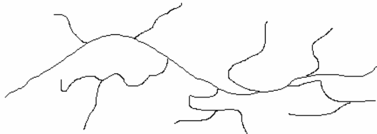
A molecule of branched polyethylene, or LDPE
