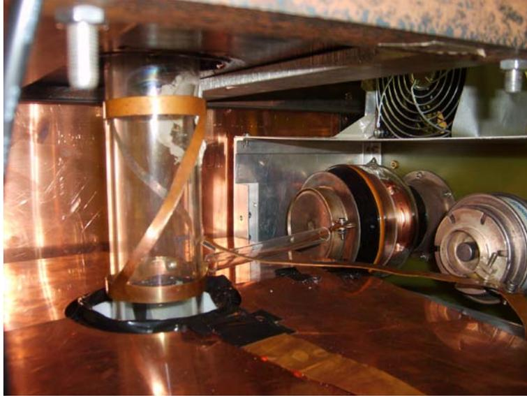
**Figure 2.11.** Picture of  $m = +1$  helical antenna system used in CHEWIE. Also shown are the capacitors in the matching box and the fan used to keep the antenna cool during plasma production. The copper sheet at the bottom is to reduce rf coupling from the antenna to the electromagnets.
