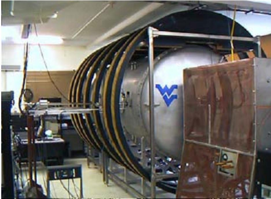
**Figure 2.1.** HELIX (foreground) and LEIA (large aluminum chamber). HELIX resides inside a Faraday cage for rf shielding. The large electromagnets surrounding LEIA are approximately 3 m in diameter. The figure is adapted from Ref. [57].
