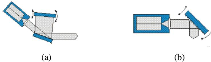
**Figure 3.19.** Two commonly used diode laser external cavity resonators. (a) Littman/Metcalf configuration. (b) Littrow configuration. The figure is adapted from Ref. [13].
