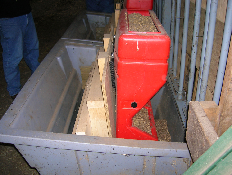
Figure 2. Modifications to GrowSafe® feed node with Kane® nursery feeder. The Kane nursery feeder was placed within the feed node to monitor feed disappearance. The feed node was modified for goats and sheep since the animals could not reach to the bottom of the node. The plywood front prevented multiple animals from feeding at one time.
