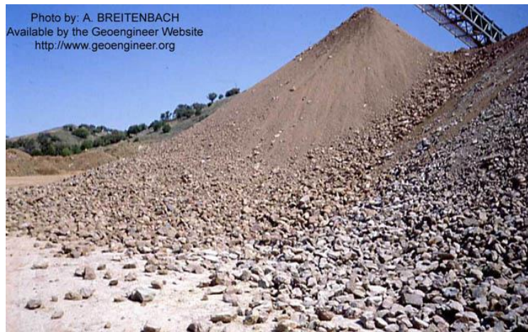
Figure 2-3 Segregation in the aggregate stockpile (Geoengineer, 2014)
