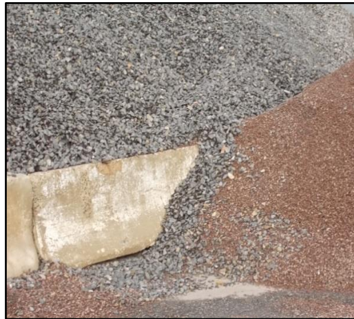
Fair separation, barrier in place but spillage observed (Project Id 34)
