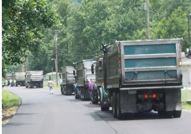
Figure 2-16 End dump trucks
