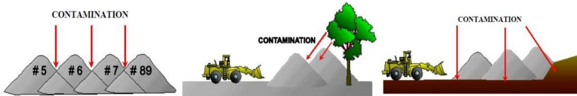
Figure 2-1 Contamination in the aggregate stockpile (GDOT, 2012)
