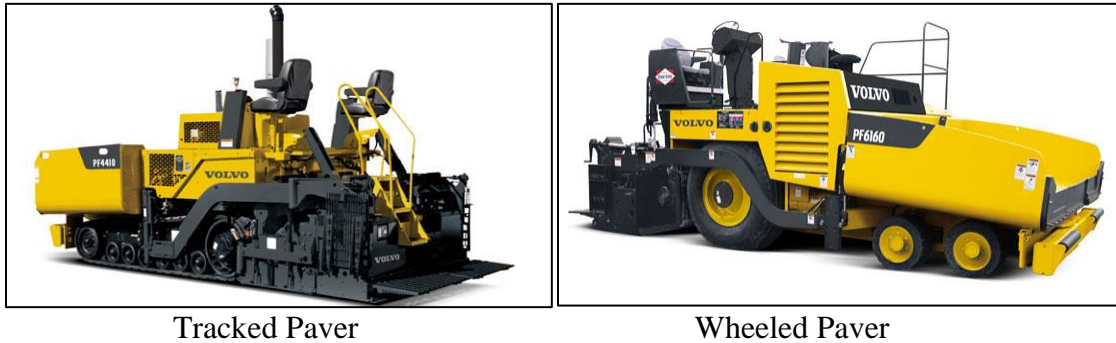
Figure 2-23 Tracked and wheeled paver (Volvo Construction Equipment, 2014)
