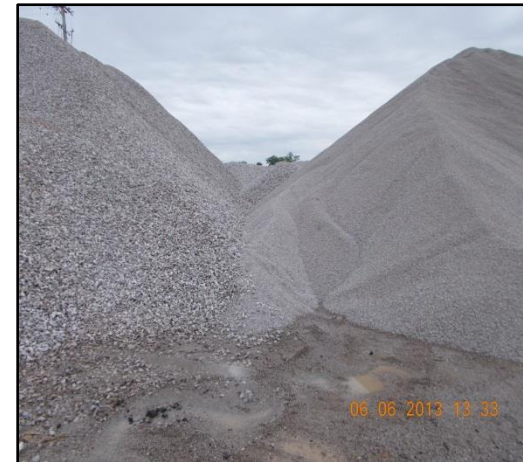
Poor separation (Project Id 142)
