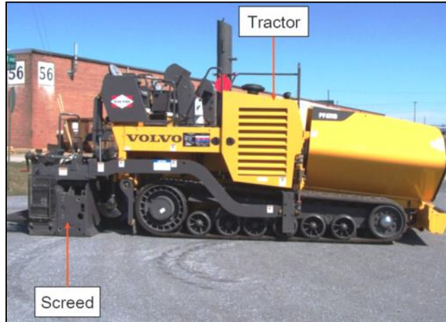
Figure 2-24 Tractor and screed in paver (Volvo Construction Equipment, 2014)
