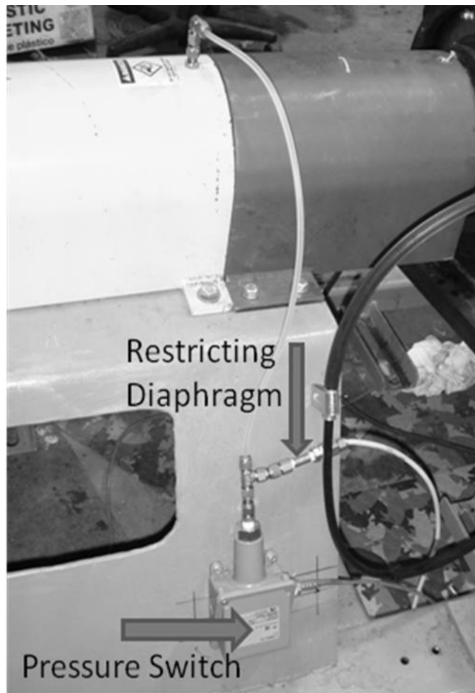
Figure 24 - Pressure Switch for Automatic Shut Off System
