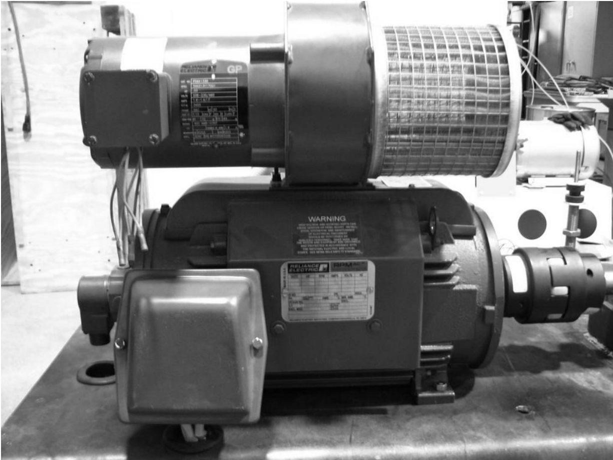
Figure 13 - Reliance Dynamometer Motor and Blower
