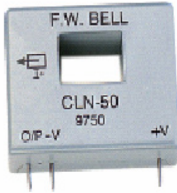
Figure 4.4: CLN-50 Current Sensor [37]
