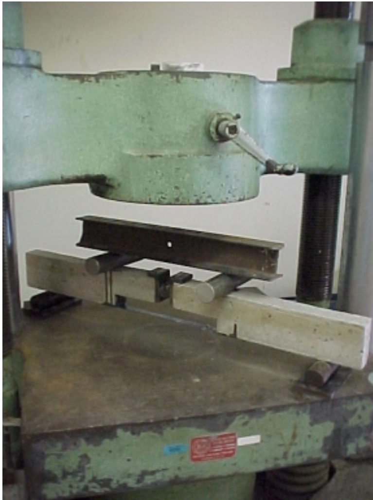
Figure 4.14 Test set-up for Beam Specimens
