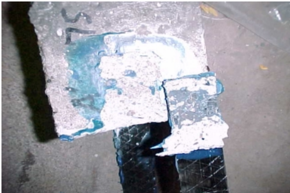
Figure 5.39 Concrete Remaining on Strip Where Strains are the Highest
