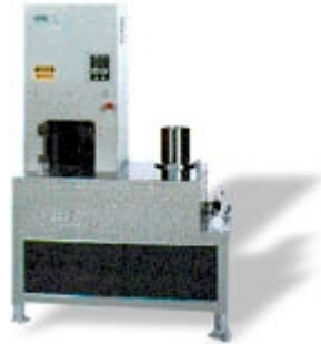
Fig. 2.1 Superpave Gyrotory Compactor
