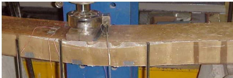
(c) facesheet-core debonding
