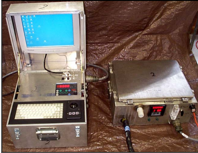
Figure 10 Data Acquisition (left) and Sample Conditioning and Analysis Systems (right) of MEMS.
