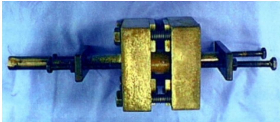
Figure 3.10 The test fixture with the bone specimen.
