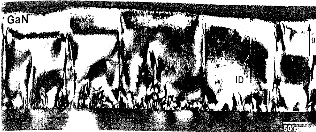
Figure 6.3 Dark field TEM image of sample 9571 (AFM image shown in figure 6.2a). 'ID' denotes an Inversion Domain. The remaining defects are non-edge type dislocations. (Photo courtesy of Dr. Linda Romano, Xerox PARC)
