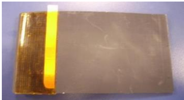
Figure 16: Covered electrode with excess dielectric towards the leading edge
