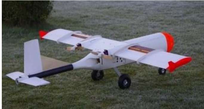
Figure 8: UAV with DBD on partial span [43]
