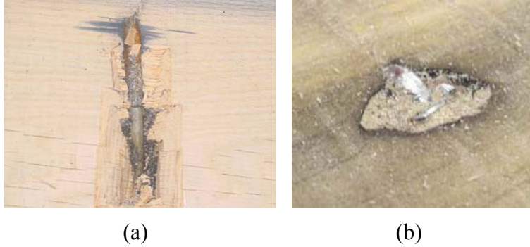
Figure 1-3 Embedded metal in wood (Agrawal 2005)
