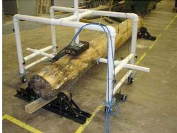
Figure 2-6 Antenna configuration for Log1 (Agrawal 2005)
