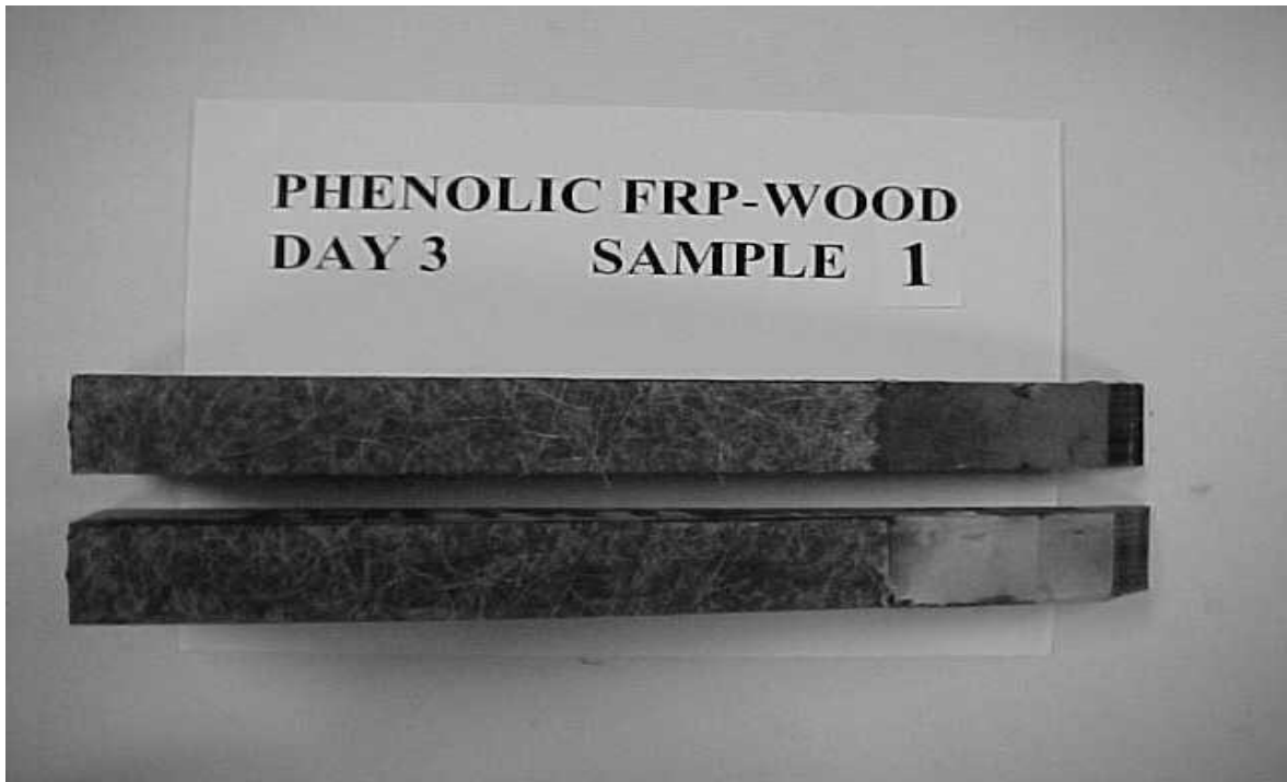
Figure 6.6. Fractured faces of Phenolic FRP-wood cycle 3 specimen #1 (Day 3-1)
