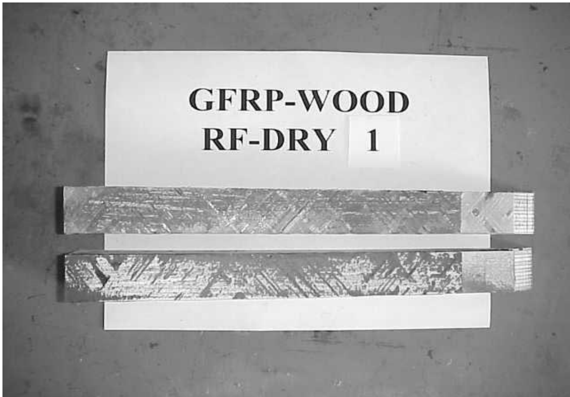
Figure 5.30. Fractured faces of Epoxy FRP-wood/RF/dry specimen (RF-DRY 1)
