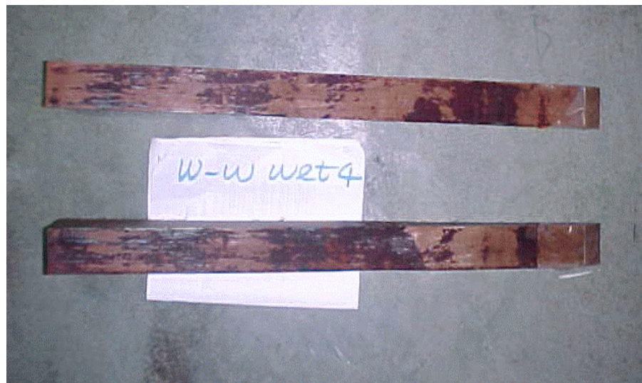
Figure 5.18. Fractured surface of wood-wood/wet specimen
