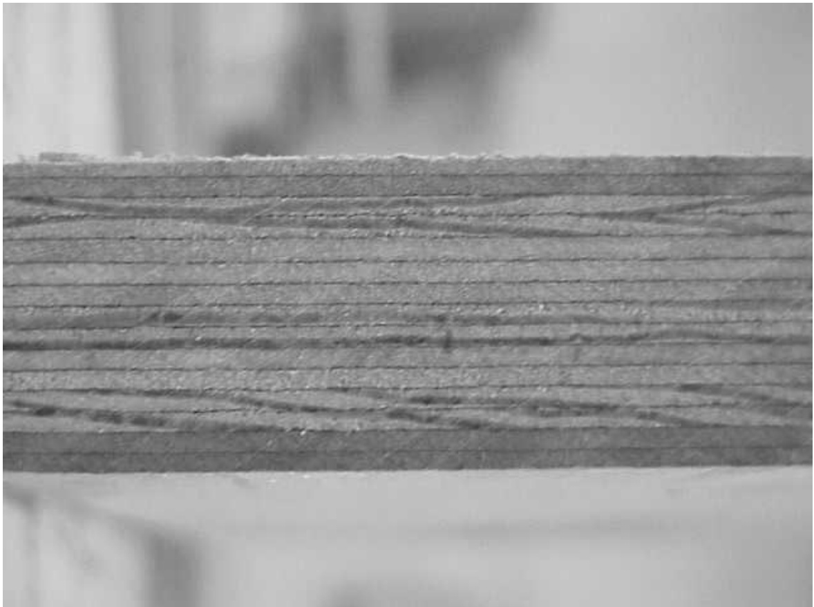
Figure 5.1 Lay-up of Linear Veneered Lumber (LVL)
