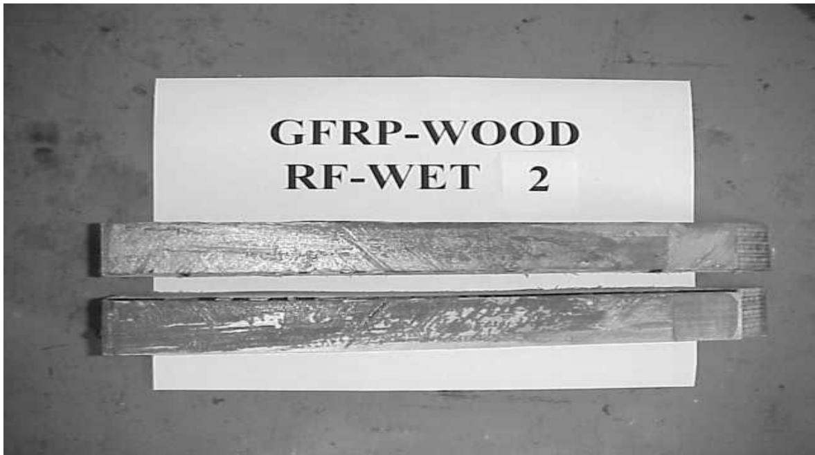
Figure 5.34. Fractured faces of Epoxy FRP-wood/RF/wet specimen (RF-WET 2)
