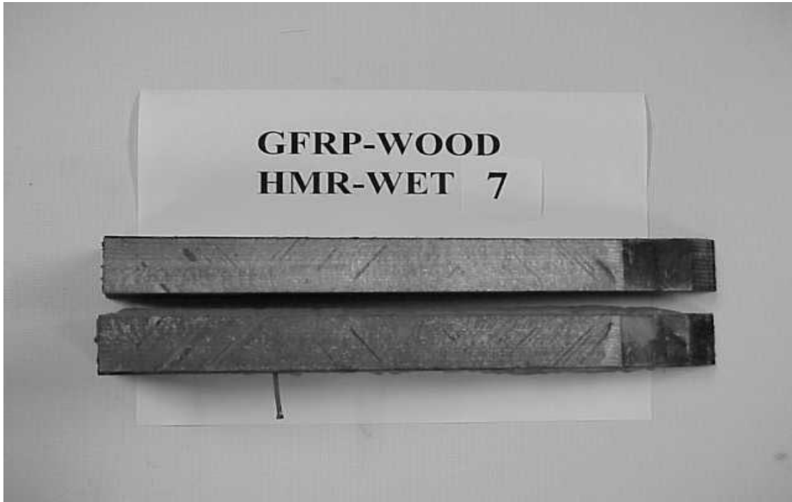
Figure 5.32. Fractured faces of Epoxy FRP-wood/HMR/wet specimen (HMR-WET 7)
