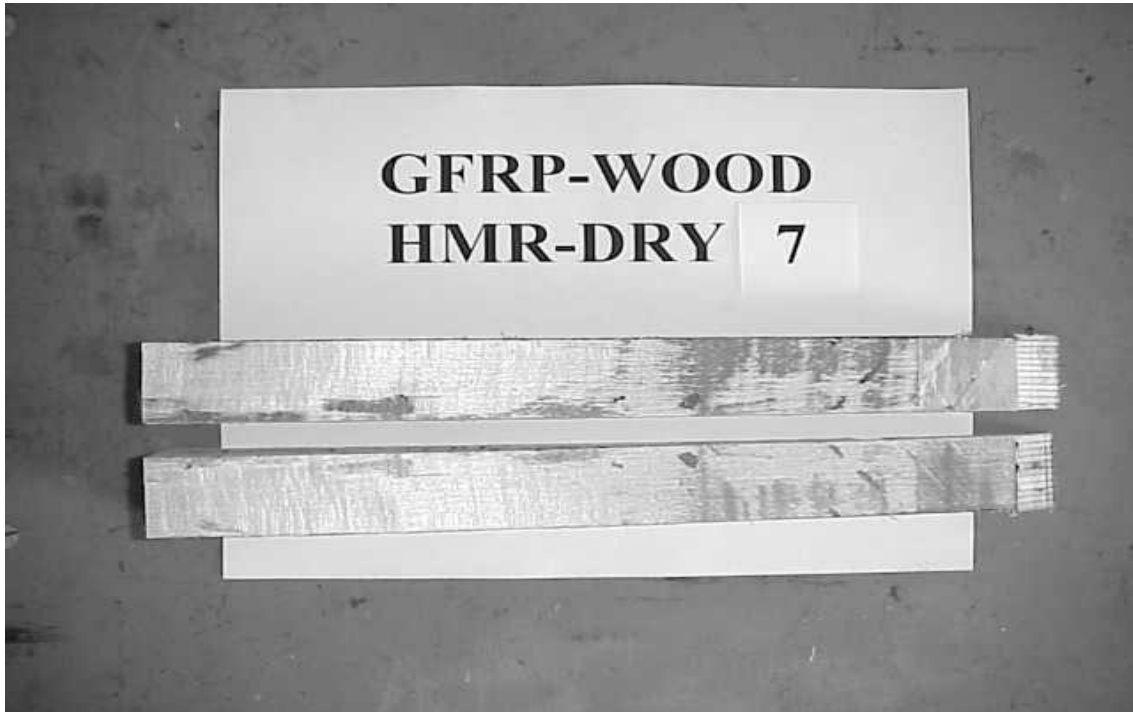
Figure 5.28. Fractured faces of Epoxy FRP-wood/HMR/dry specimen (HMR-DRY 7)
