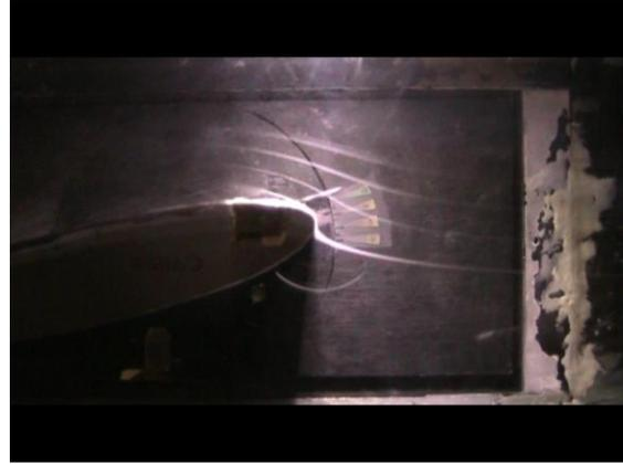
**d) Airfoil at 12 degrees angle of attack with separation and stall**
