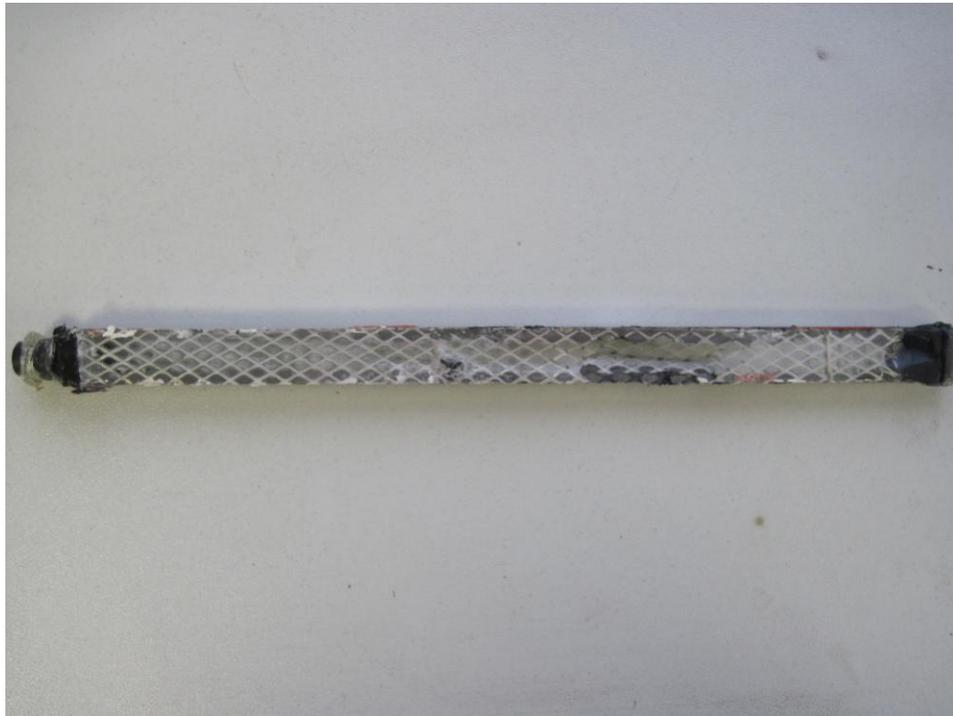
**Figure 6.5: Completed dynamic roughness apparatus**
