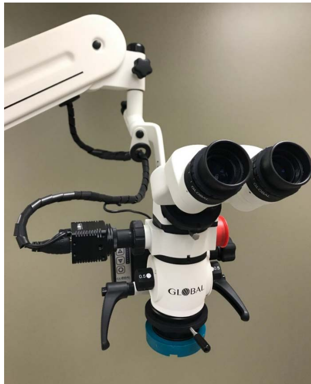
Figure 14: Dental operating microscope used for instrumentation and obturation of samples (Global Surgical Corporation, St. Louis, MO).
