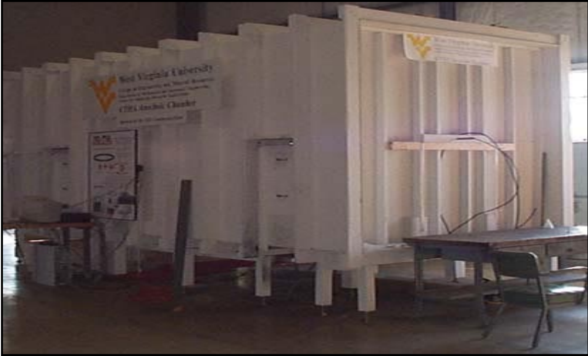
Figure 4.1b Anechoic chamber at West Virginia University
