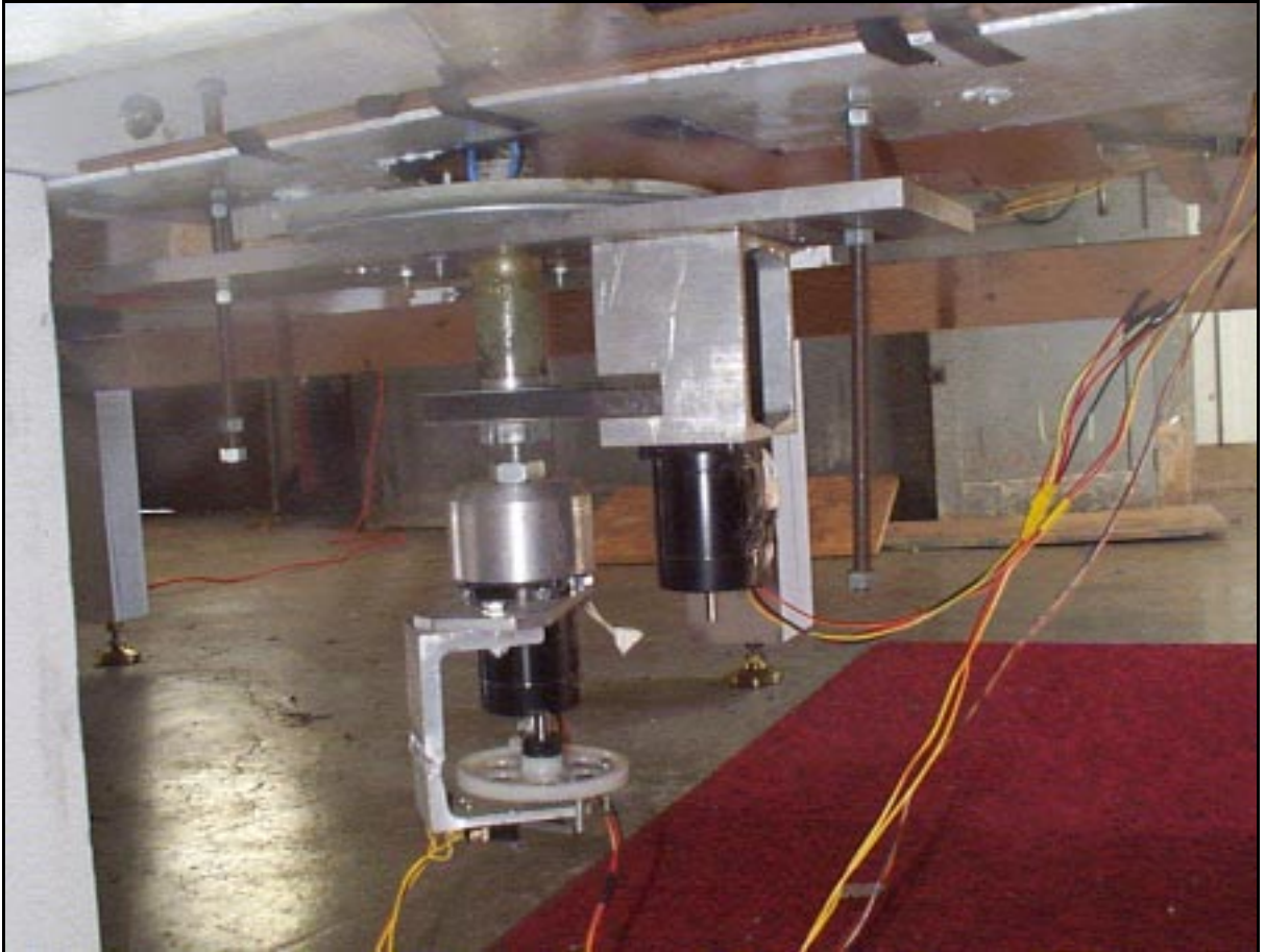
Figure 4.9 Motor and limit switch assembly on the rotator
