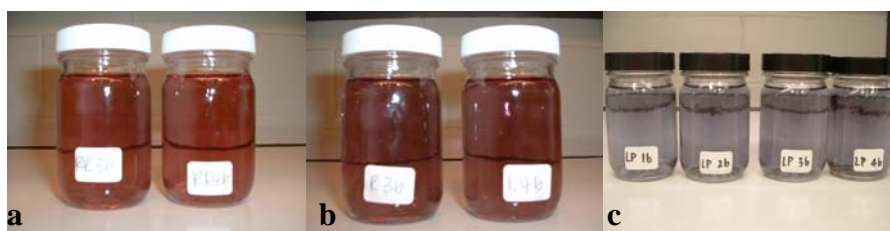
Figure 5.19. Reactions of RR, R, and LP extracts with \text{KAuCl}_4 showing final products diluted 20X for (a) RR, (b) R, and (c) LP.
