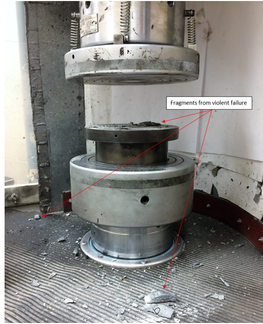
(b) Diabase Core Post-UCS Failure
