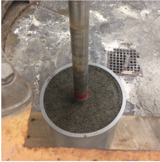
(a) Drilling a Bolt Hole in 10%wt. Regolith
