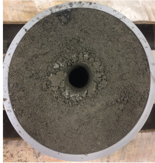
(b) Completed Bolt Hole in 5%wt. Regolith
