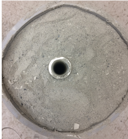
(c) Modified Bolt Hole Preparation for 0%wt. Regolith
