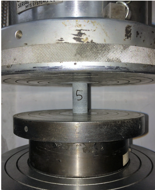
(a) Diabase Core Prepared for UCS Testing
