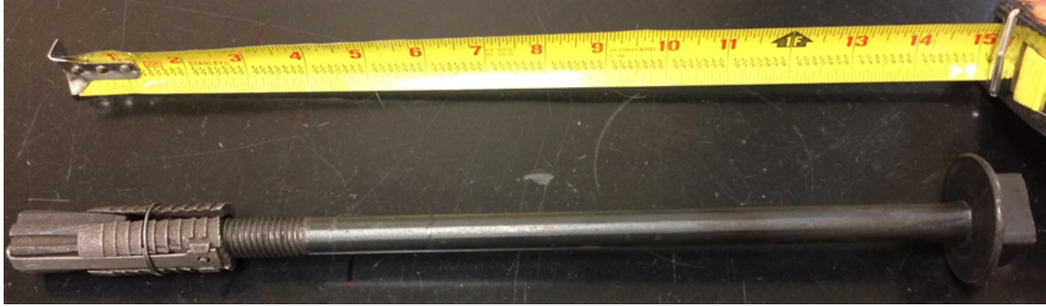
(a) Point Anchor Roof Bolt
