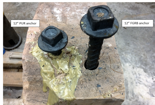
(b) Bolts Installed In The Sandstone Boulder
