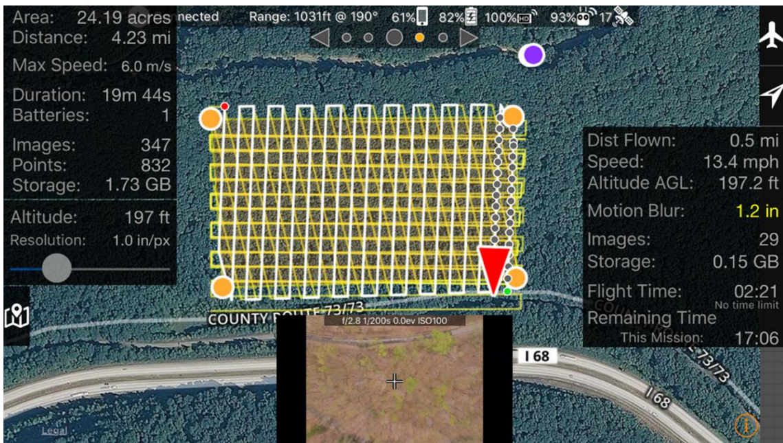
Figure 3. 'Map Pilot' application on-screen display while UAV is in flight. Still images are shown in display in bottom center of screen. UAV location and flight direction represented by red triangle, orange circles represent corners of area of interest and grey circle represent locations of images that have already been acquired.
