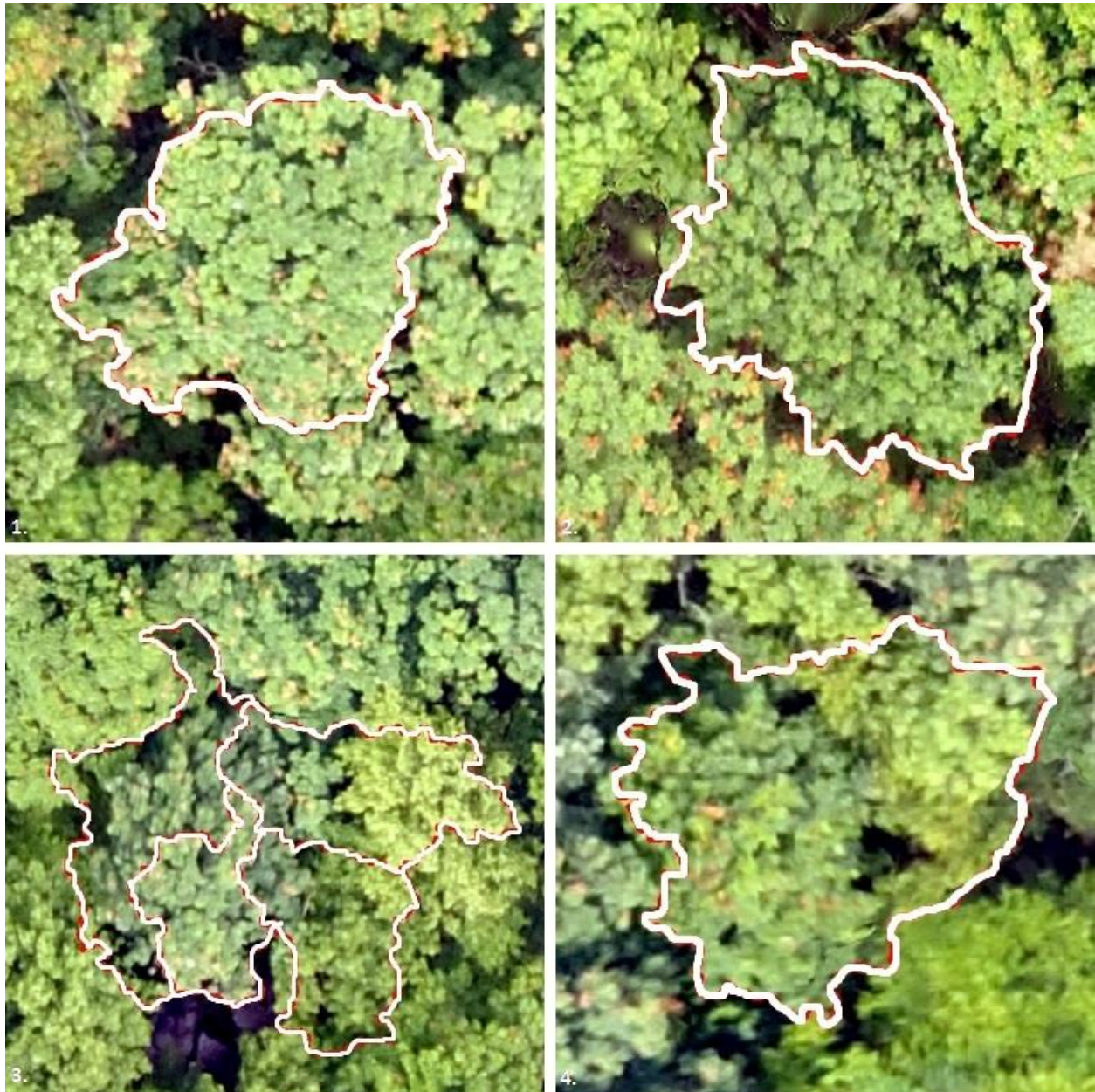
Figure 13. Counterclockwise from the upper left: (1) Correctly segmented tree crown that would be considered a success; (2) correctly segmented tree crown that would be considered a success; (3) Over segmented tree crown that would be considered a failure; (4) Under segmented tree crown that would be considered a failure.
