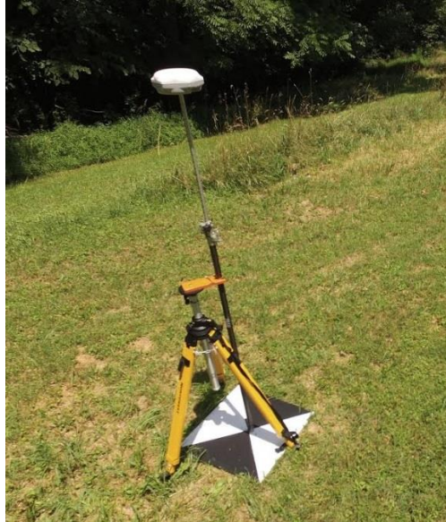
Figure 8. iGage X900S-OPUS GNSS static GPS receiver and 4 ft 2 black and white plywood target deployed at ground control point location. The static receiver was moved to each GCP location while the targets remained for visibility in aerial imagery.
