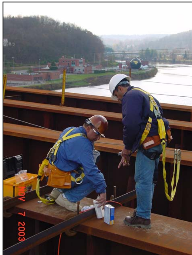
Figure 4.28 Mounting Strain gages on Steel Girders of Mid-span 2
