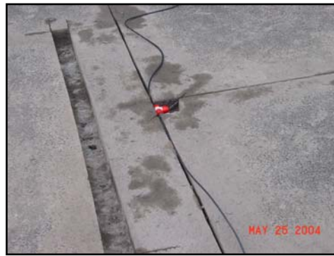
Figure 4.18 Weigh In Motion System at the Bride Entrance
