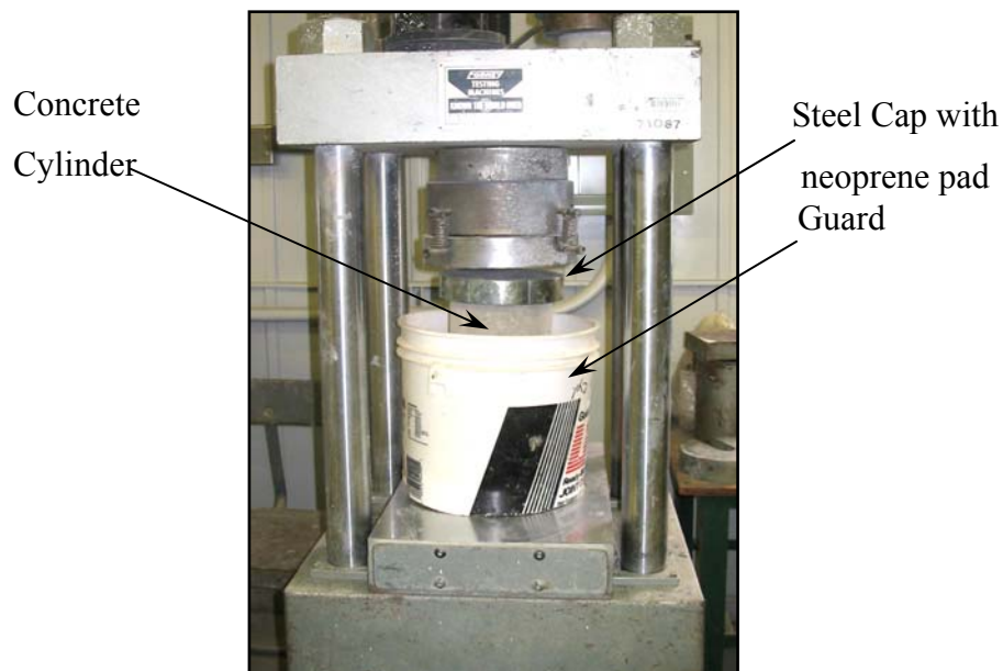
Figure 3.9 Testing of Compressive Strength of Concrete
