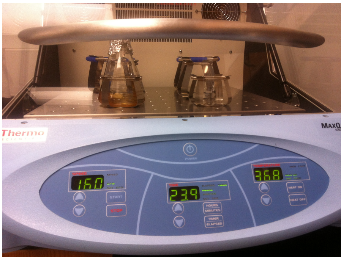
Figure 21: Heated shaker machine used for sample incubation before plating
