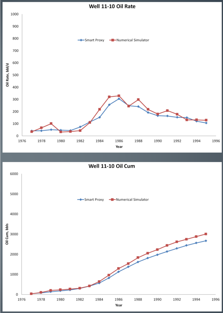
Figure 8.41: Phase three well 11-10 oil production profile
