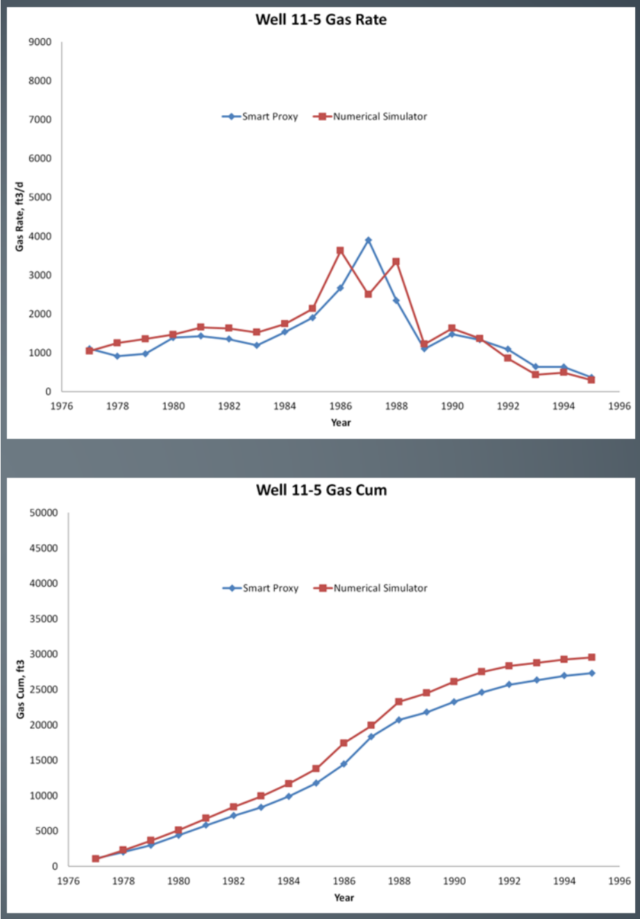
Figure 8.33: Phase three well 11-5 gas production profile
