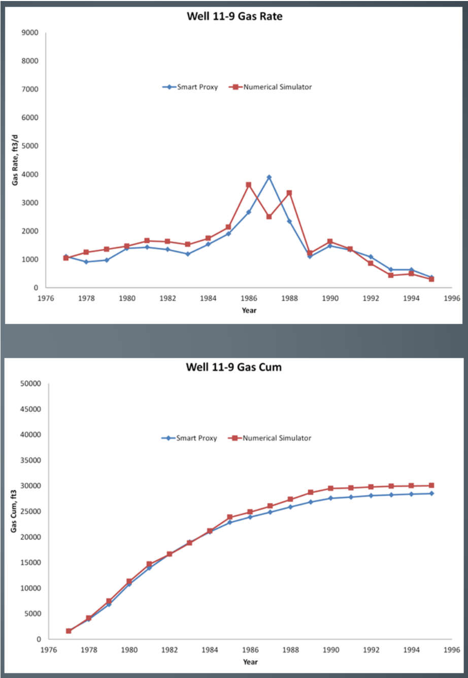
Figure 8.39: Phase three well 11-9 gas production profile
