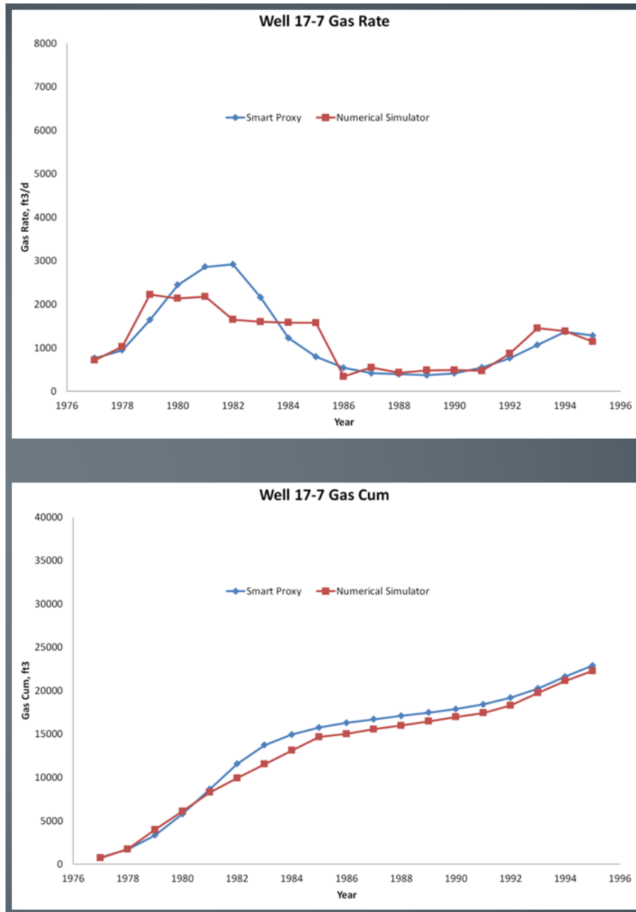
Figure 8.45: Phase three well 17-7 gas production profile
