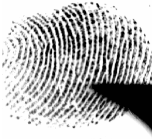
Figure 50. Shadowing Effect on Fingerprint Sample
