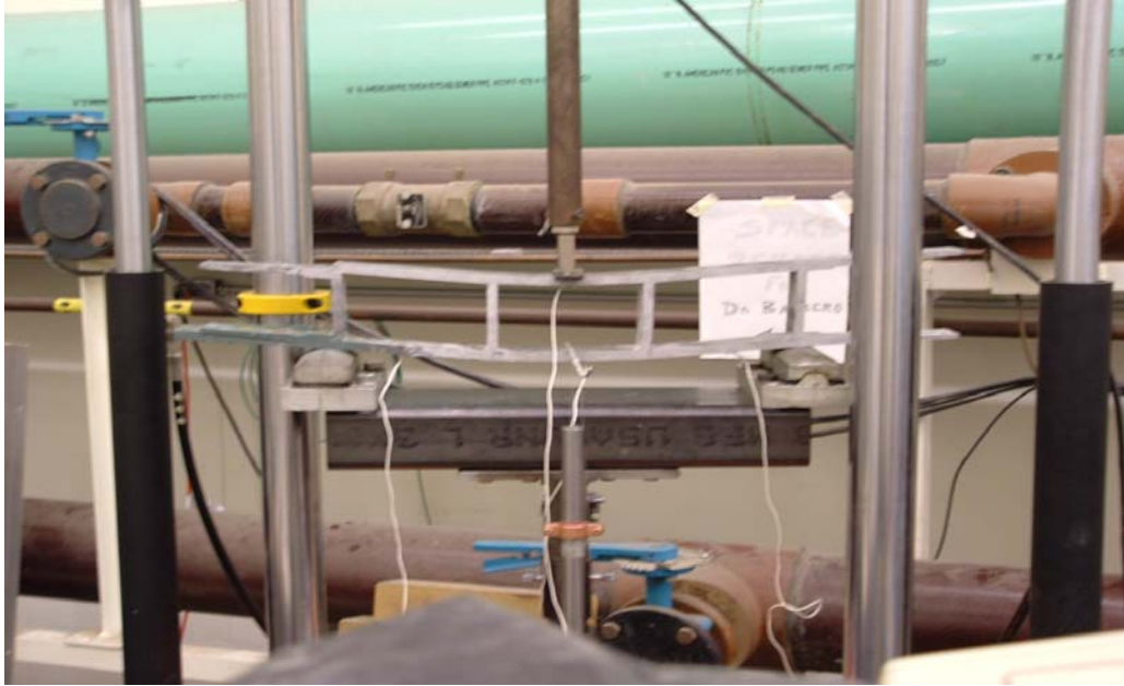
Figure 4.35 Loaded bending specimen
