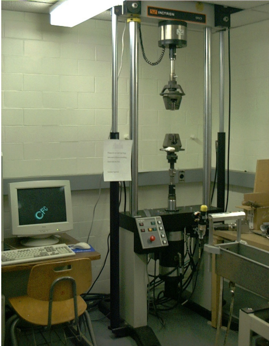
Figure 4.1 INSTRON 8501 Loading Frame, Load Cell, and Actuator
