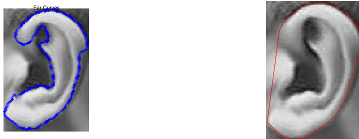
Figure 63: a) ear extracted curves; b) convex hull separating the segmented ear from background
