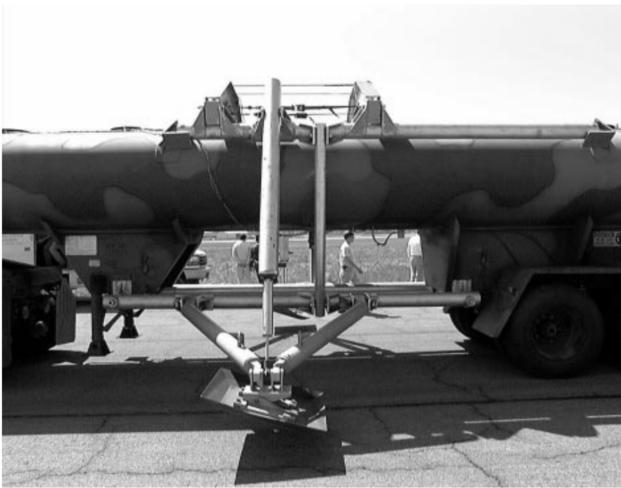
Figure 3.2: Artificial trailer outriggers to prevent vehicle rollover during tests
