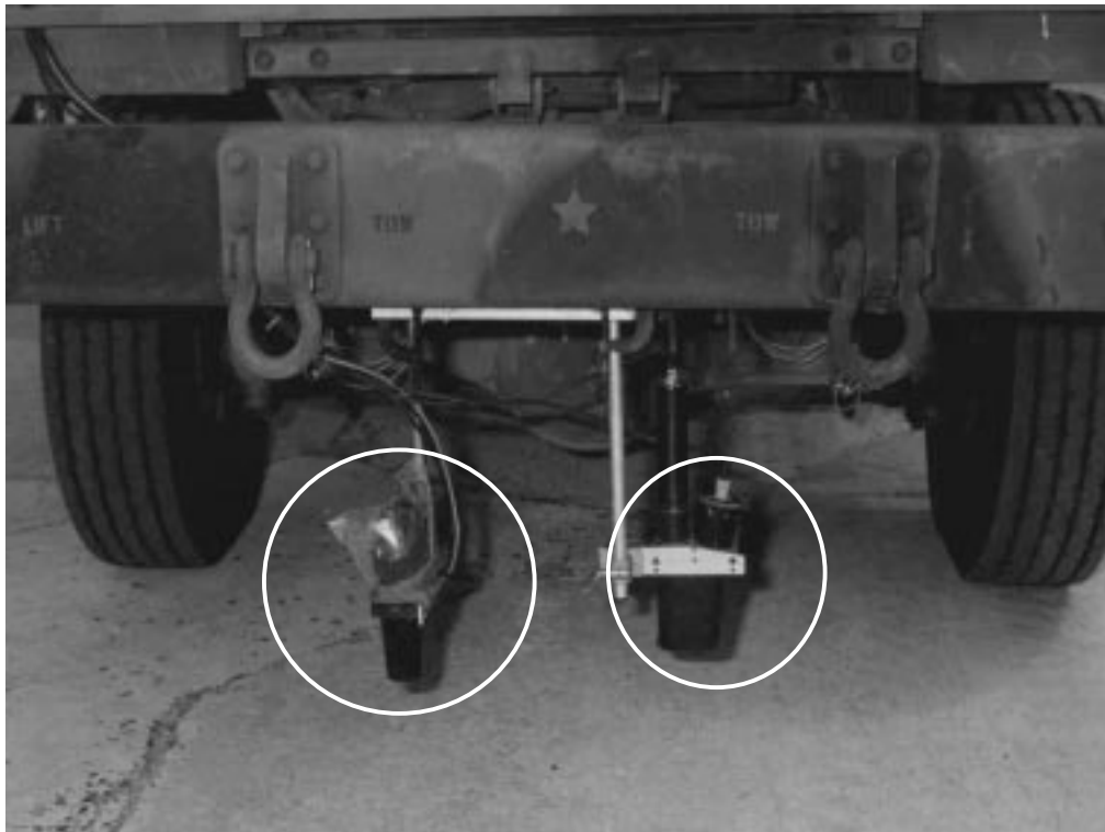
Figure A.4: Oscillation Gyrometer to measure the Yaw rate of the tractor and lateral speed sensor
