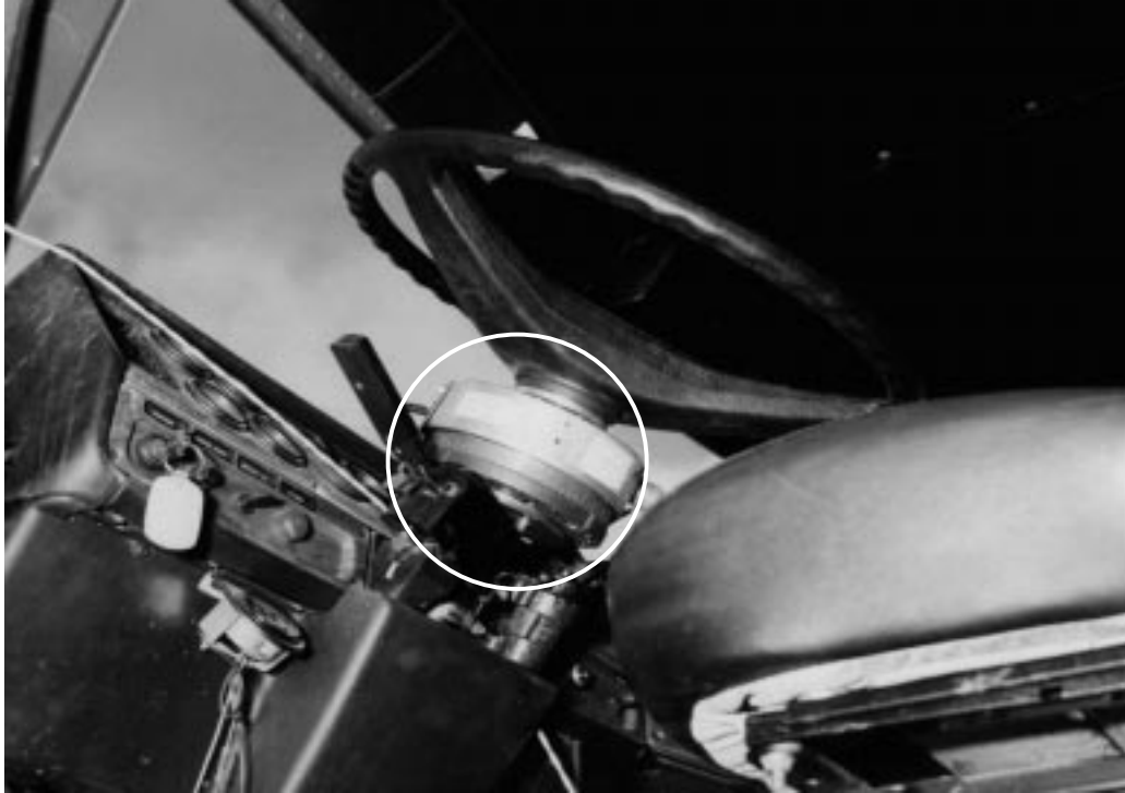
Figure A.8: Circular dial to measure the steering angle and hence the slip angle of the tires can be determined (device was not needed in this study but could be used later)
