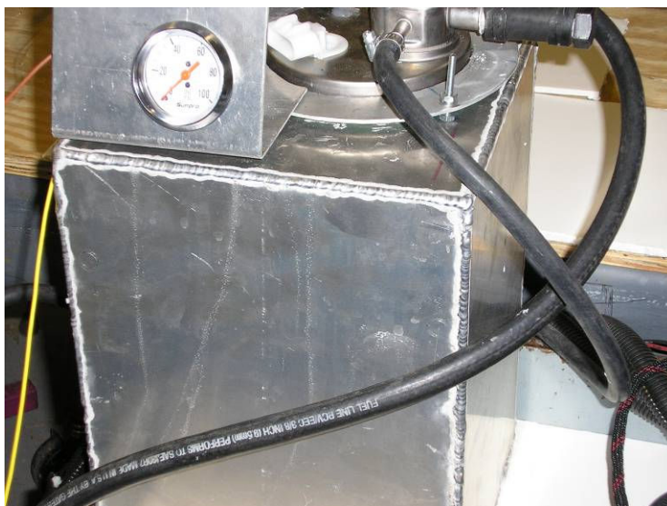
Figure 3.3 Urea Storage Tank with Fuel Line and Pressure Gauge
