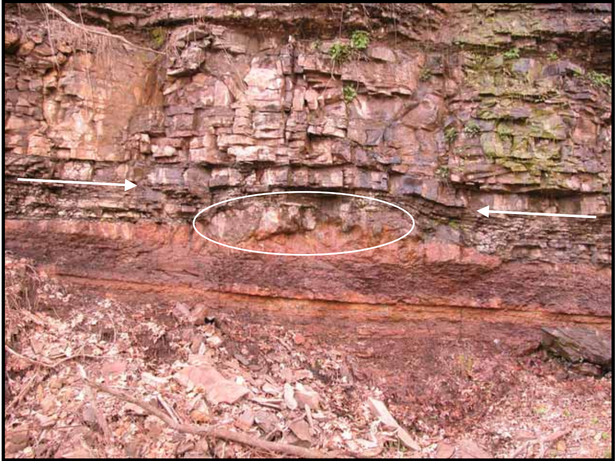
Figure 30. Photo ID #0572: Photo shows sharp basal contact (indicated by arrows) of Unit 34 at Rowlesburg. Note the large convex “conglomeratic bar” at the base.
