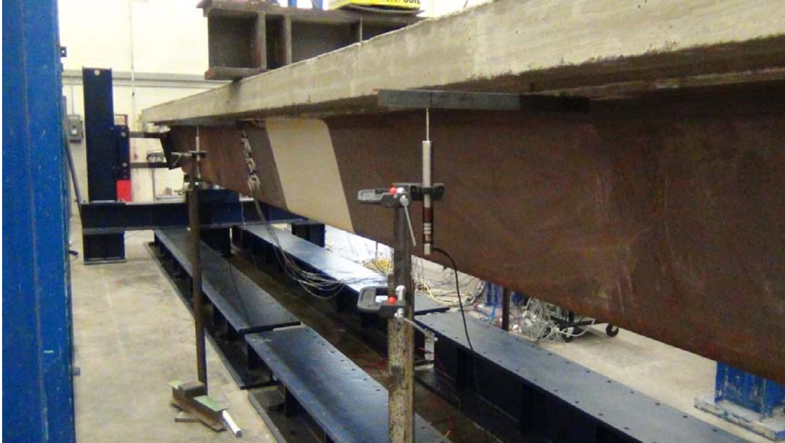
Figure 4.14: LVDTs Measuring Vertical Deflection
