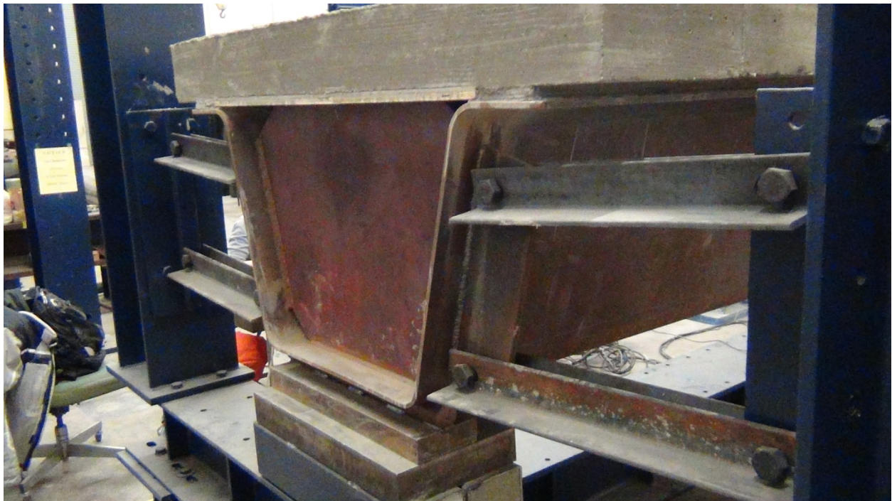
Figure 4.4: In-Place View of Typical Support Conditions
