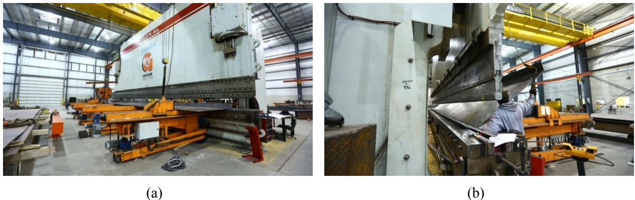
Figure 4.5: Forming Process, (a) Press Brake, (b) Bending of Specimen's Top Flange.
