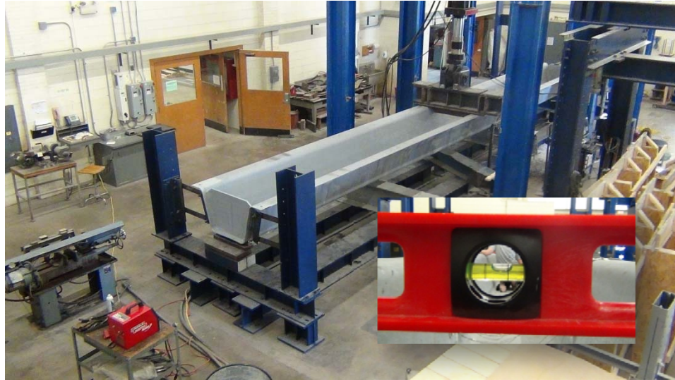
Figure 6.13: Galvanized Girder Test (Initial Twist Present)
