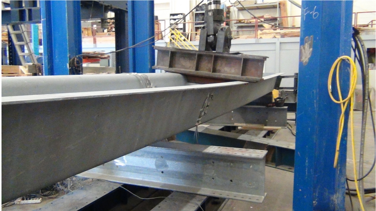
Figure 4.18: Typical Failure Mode for Noncomposite Specimens
