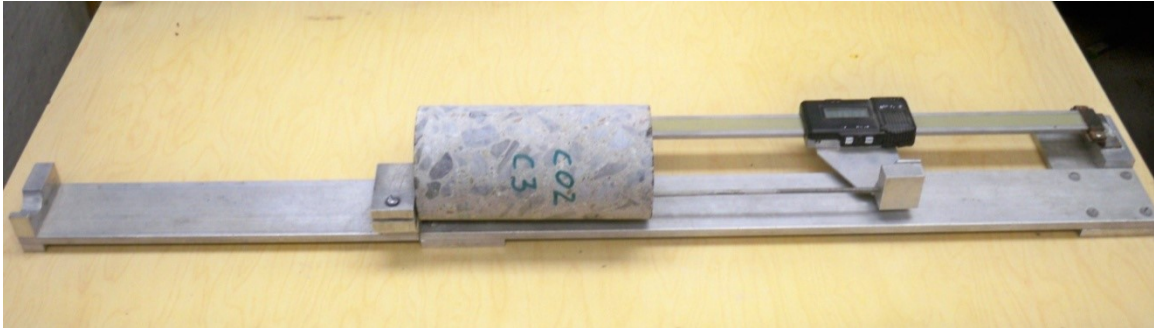
Figure B-8 Sliding digital caliper used to measure length of core specimens.
