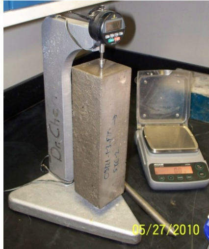
Figure B-6 Length comparator with reference bar, as used for shrinkage and elongation monitoring.
