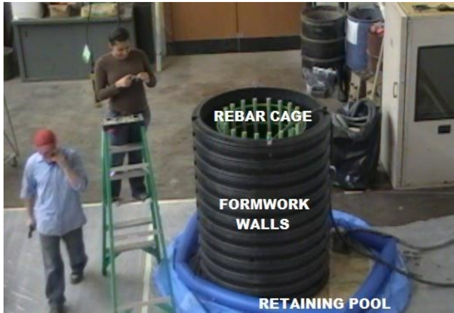
Figure 3-6 Picture of laboratory trial caisson formwork and setup.
