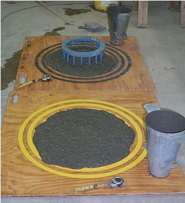
Figure 2-2 Photo of slump-flow (bottom) and J-Ring (top) patties after removal of the Abrams cone.
