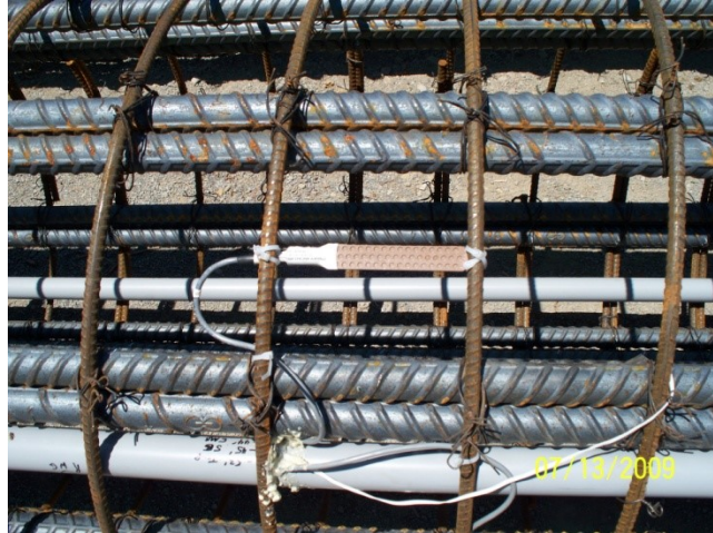
Figure 3-22 Concrete embedment strain gage, before and after affixing to caisson rebar cage.
