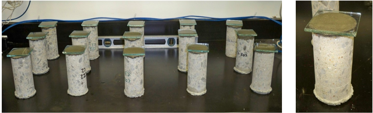
Figure 3-16 Trial caisson compressive cores during mortar capping.
