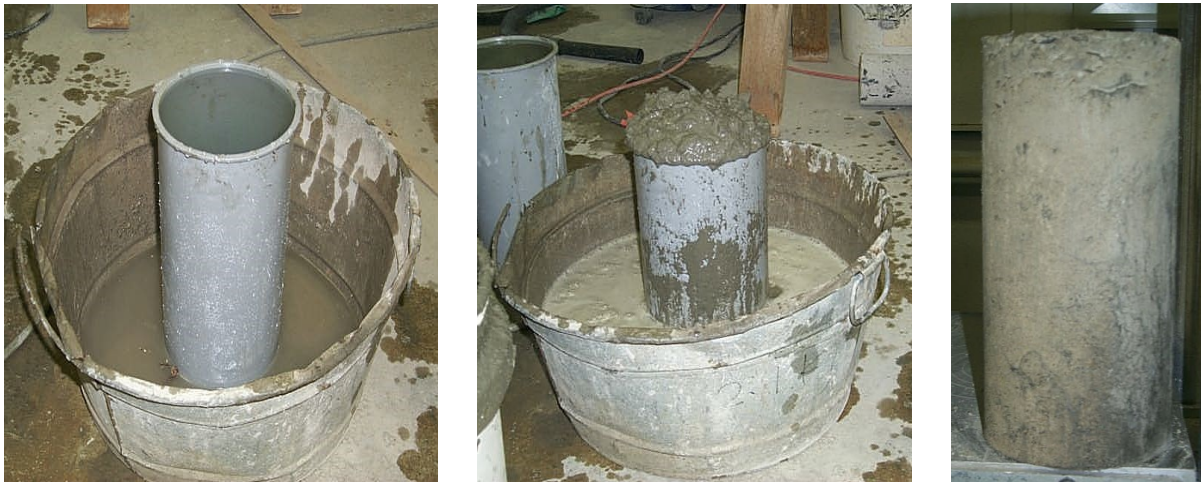
Figure 3-4 SCC specimen cast into water-filled cylinder mold.
