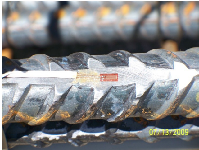
Figure 3-23 Foil strain gage, before and after mounting on steel rebar (before protection).
