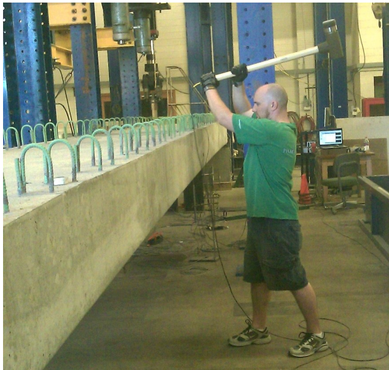
Figure 4-62 Delivery of impact during modal analysis of test beam using instrumented sledgehammer.
