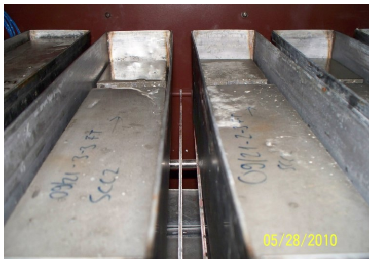
Figure B-5 Configuration of 3"x3"x11" specimens with blocks during freeze-thaw testing.
