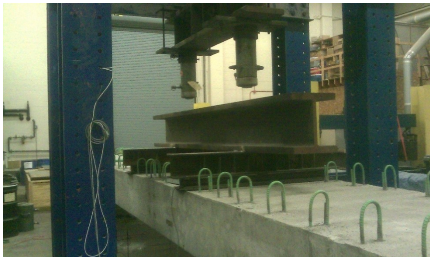
Figure 4-26 Spreader beam apparatus used for static testing of laboratory beam.
