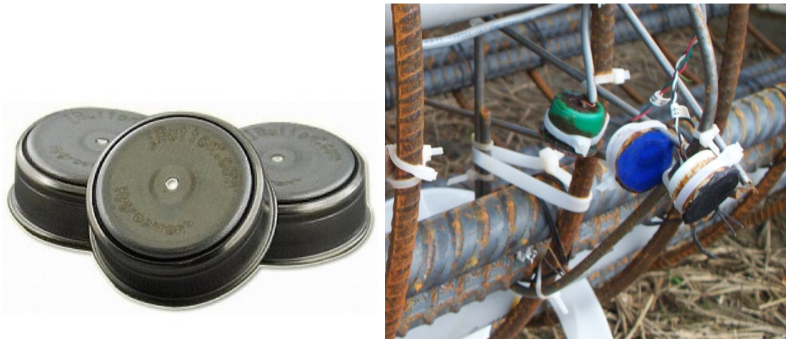
Figure 3-25 Thermal logging hygrochrons, before and after protecting and mounting on steel cage.
