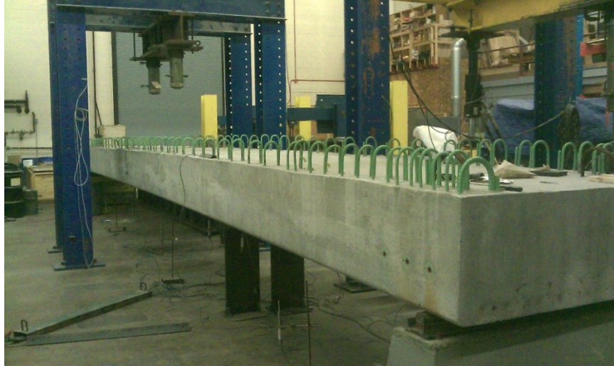
Figure 4-23 Full-scale box beam in WVU laboratories after placement on roller supports.
