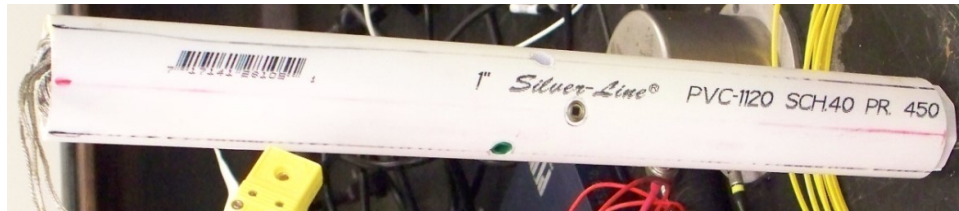
Figure 3-36 Probe for Infrared Thermal Integrity Testing.
