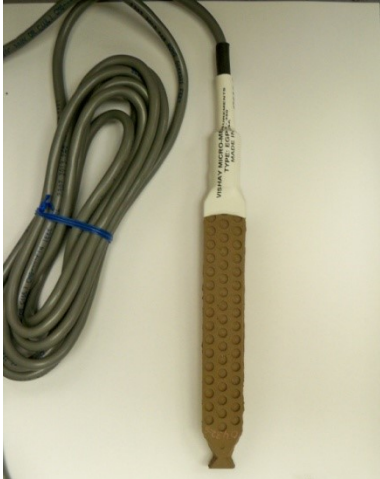
Figure 3-22 Concrete embedment strain gage, before and after affixing to caisson rebar cage.
