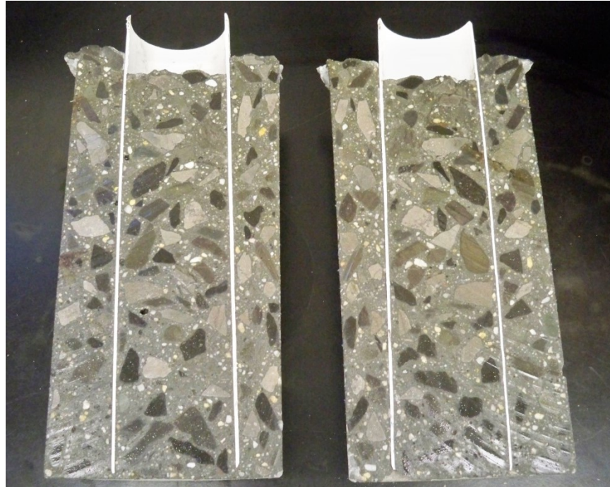
Figure 3-5 Aggregate distribution in 6"x12" cylinder after "fresh core" tube (4"dia.) insertion into 1.5-hour-old SCC.
