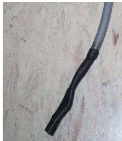
Figure 3-24 Analog temperature sensor, before and after attaching wire and protection.
