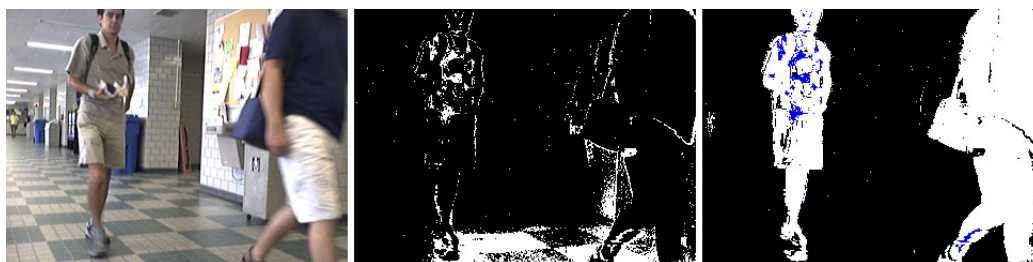
Figure 3-5: Shadow detection error corrected by spatial information.
