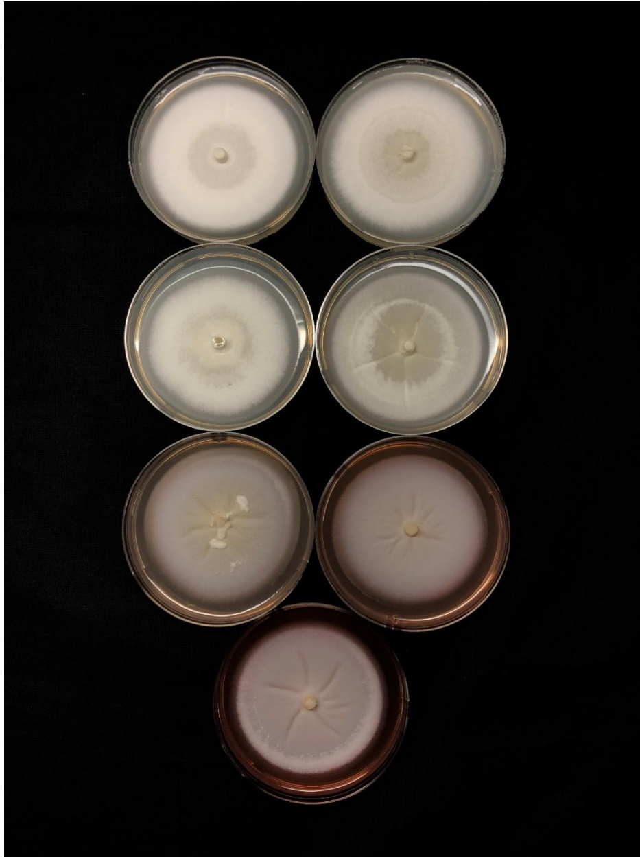
Figure 4-5: Seven treatments of gradually increasing iron concentrations in the form of Sequestrene 138 added to potato dextrose agar plates with pure cultures of V. nonalfalae placed in the center of the plate after being excised with a sterile 4mm cork borer. Measurements of growth, conidial production and viability occurred after 3 weeks of growth at ambient room temperature.
